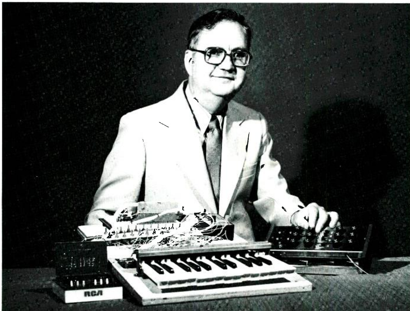
Author with his Combo. At left is the RCA COSMAC Microtutor; at center (front to rear) are the keyboard, interface, and attenuator; synthesizer at far right.
