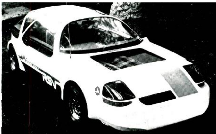
Fig. 5 — Latest version of Research Safety Vehicle. Radar will be fitted under rectangle on right side of hood.
