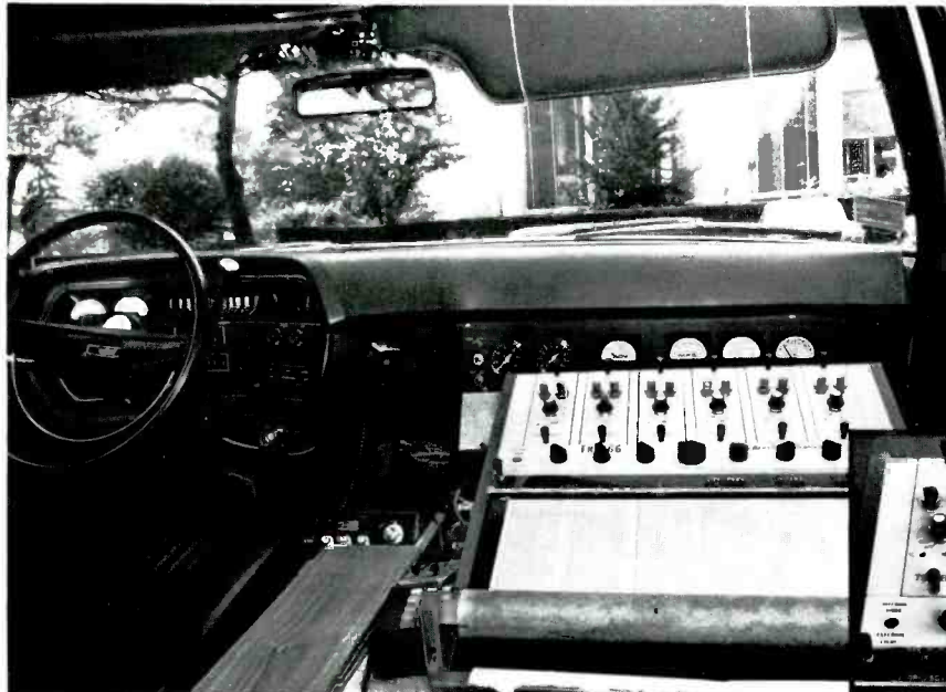
Instrumentation includes numerous gauges, including spark advance and gasoline mileage. At right, strip-chart recorder displays fuel-flow parameters. Note difference between gas flow in carburetor (far left) and gas flow in line (second from left).
