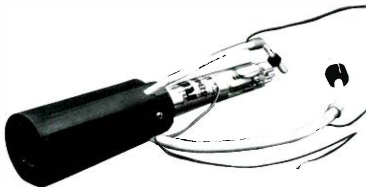
Fig. 2 — The I-SIT tube — an image intensifier tube coupled by means of fiber optics to a SIT camera tube.
