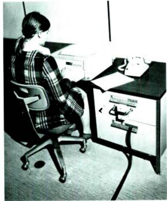
Fig. 2 — Part programs are prepared by perforating paper tapes to be used in controlling part production.
