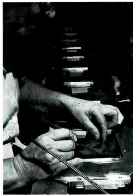
Fig. 16—The outer shield being placed back in position with a hand-soldering operation being performed to form a continuous shielded junction. The cable is positioned in the tool as shown and is immediately passed through the potting operation to form a final matrix junction with strain relief provisions.
