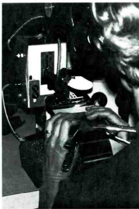
Fig. 14—Another view of the welding process. Here connection is being made to one of the 2½-inch wafer/pin combinations. The wafer has built-in provision for accepting the laminated conductor strips and positioning these under the connecting pins while maintaining all conductors on the 0.05-pitch. Welding is performed through a slot in the wafer which is sealed with an epoxy potting compound after the welding operation.
