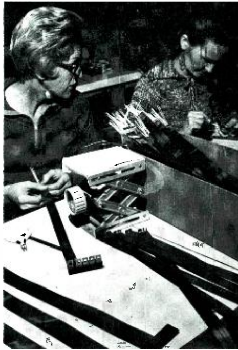
Fig. 12—Typical operation in preparation of ribbon cable for mating with the connecting wafer. Shown is a DC power conductor, with the ribbon being connected by weld terminations to a number of parallel wires which will in turn be welded to the connecting pins.
