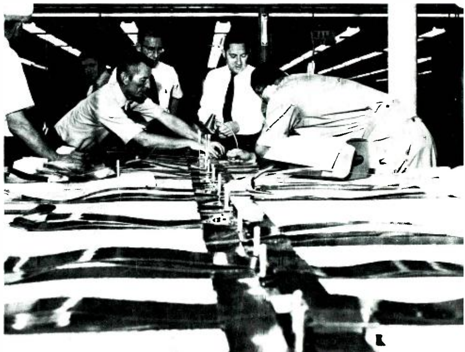
Fig. 17—The completed assembly being readied for shipment. The cable is placed on a plywood board and secured against travel stresses as indicated. The board holds the cable in position for a direct transfer to the rear flanges of the array, with consequent saving in assembly line.
