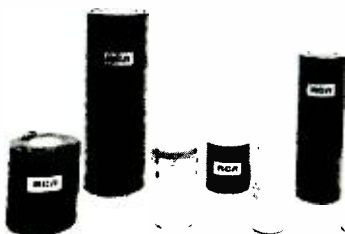
Fig. 2—Image intensifiers. Left to right: 25-mm second generation, potted; 25-mm first generation, potted; 25-mm second generation, unpotted; 18-mm second generation, potted; 18-mm second generation, unpotted; 18-mm first generation, potted.
