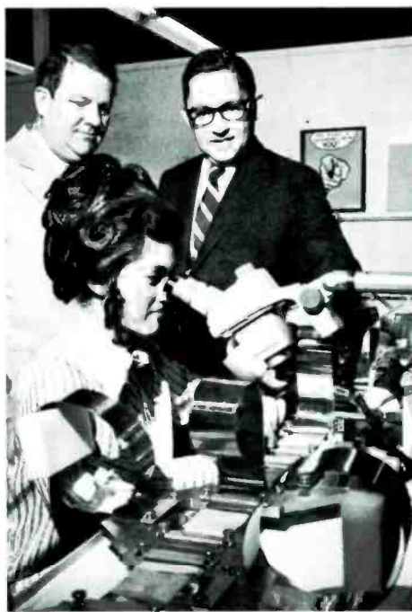
Fig. 15—The matrix-welding operation showing the ribbon cable with the outer shield stripped back and the weld junctions being performed by the flex-weld process. All junctions are later visually and electrically inspected, with 100% of all weld junctions coming under scrutiny.
