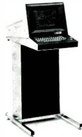
Fig. 3—Bistable direct-view storage tube in a computer display terminal. (Courtesy of Tektronix, Inc., Beaverton, Oregon.)
