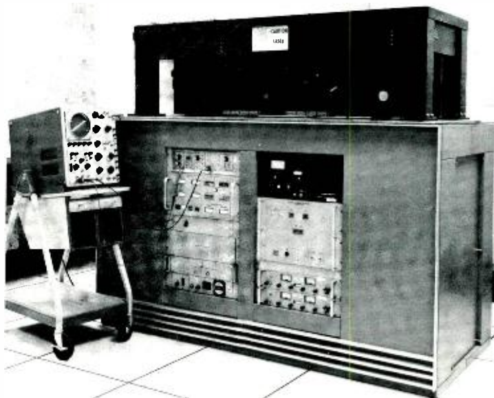
Fig. 1—Advanced Laser Beam Image Reproducer (LBIR).
