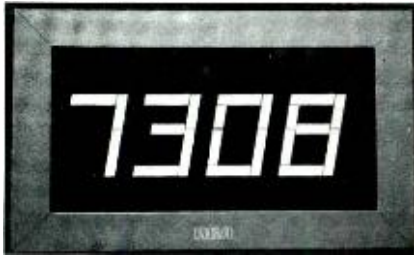
Fig. 4—RCA liquid crystal display (reflection type).
