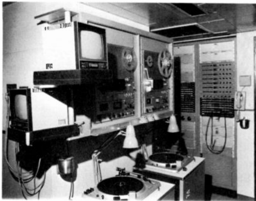
Fig. 6—Portion of the audio control equipment, including transcription turntables and tape machines.
