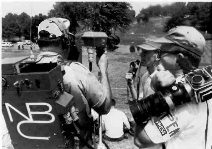
Fig. 3—Above, a portable, back rack, RF-connected camera used at Firestone Country Club in Akron, Ohio by NBC field crew.
