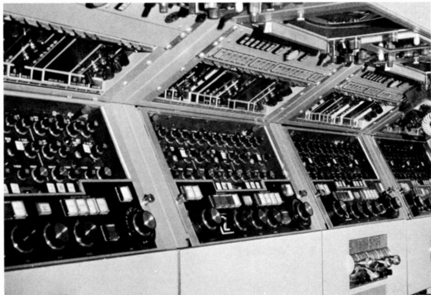
Fig. 3—Video control console; the “joystick” central control position is located in the lower right-hand corner of the photo.
