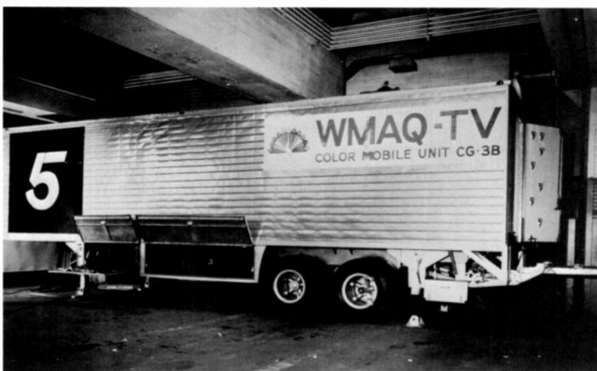
Fig. 5—CG-3B (carryall) showing hydraulic lift gate on rear. A similar gate is on the side.
