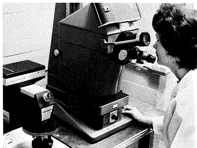
Fig. 2—The interferometer used for measuring substrate flatness.
