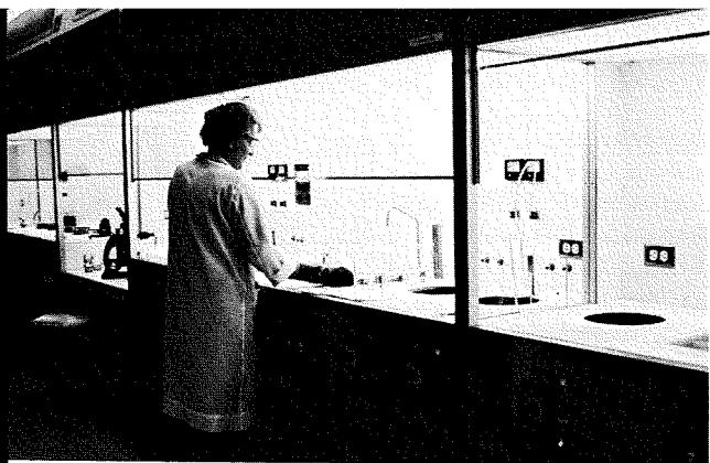
Fig. 20—Class 100 laminar-flow-hood system of environmental control.
