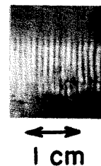
Fig. 11—Far-field interference of laser beams from two corners of CdS crystal at room temperature.
