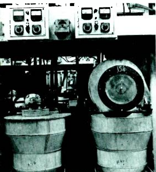
Fig. 4—One type of disc-rotating unit used to make electroformed metal master.
