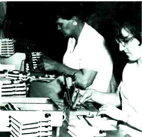
Fig. 6—SPLICING. Ends are spliced to create the endless loop of tape. A sensing foil, which actuates a head-positioning solenoid in the player, is affixed during the splicing operation. Cartridge bases delivered to these stations are prenumbered for control purposes. Each group of tapes, from the same original reel, is accompanied by a data-processing card which provides information on efficiency, quality, shrinkage, and finished goods deliveries.
