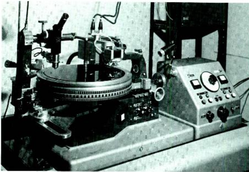
Fig. 4—Type of disk-recording lathe used in commercial disc-mastering.
