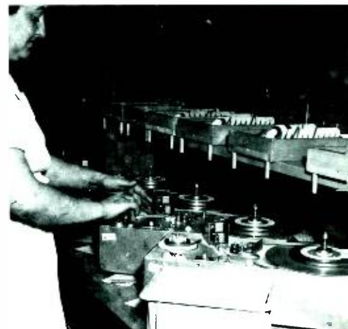
Fig. 4—BREAKDOWN OPERATION. The multiple recordings on the large reel of tape are separated into individual cartridge lengths on breakdown machines. During recording a subsonic signal is recorded after each cartridge length; this signal activates a cutter on the machine which cuts the tape automatically.
