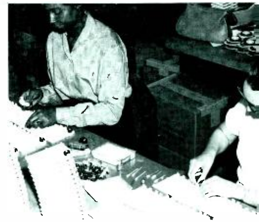
Fig. 5—PARTS SUBASSEMBLY. Except for the tape-supporting platform, parts subassembly off-line and delivered to the production lines in bulk.
