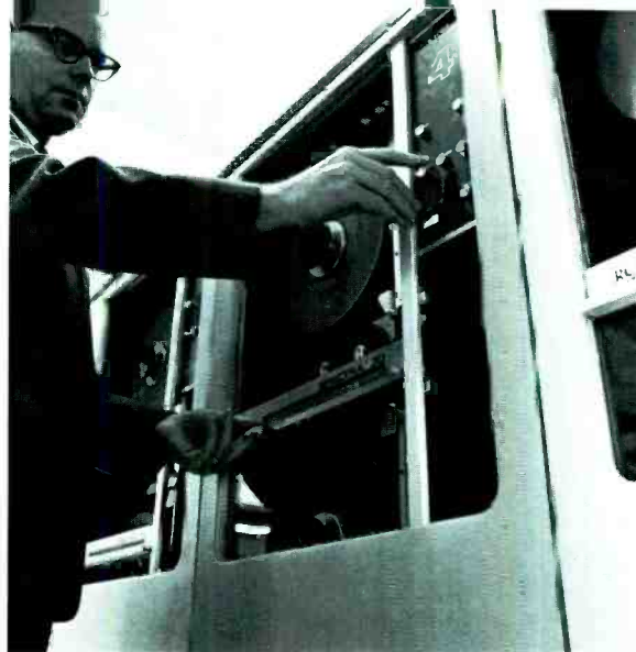
Fig. 2—RCA's Spectra 70 magnetic tape unit combines two tape drives with independent electronics. Basic speeds are 30,000 or 60,000 EBCDIC bytes or 7-level characters/sec at a packing density of 800 bits/inch, using 1/2-inch tape on 2,400-ft reels.
