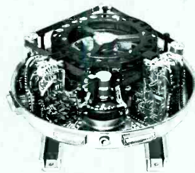
Fig. 7—Nimbus satellite high resolution infrared (HRIIR) tape recorder (top cover removed).
