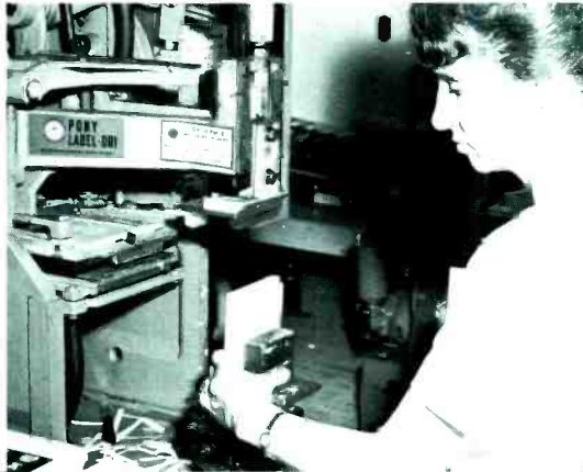
Fig. 9—LABELING. Approved runs of finished cartridges are conveyed into the packing room where two heat-activated labels are applied to each cartridge by automatic labeling machines.
