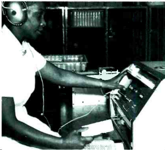
Fig. 8—LINE TESTING. In addition to constant sampling of the product on a statistical basis, the first copy from each reel of tape (which was the last to be recorded on the slave unit) is played through the splice on all programs to assure that the tape has been cut and spliced properly. Copies are also checked against sequence sheets and label copy for content assurance.
