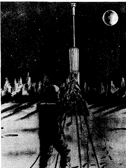
d. A protective cover (thermal shield) is removed before the reflector is deployed.
