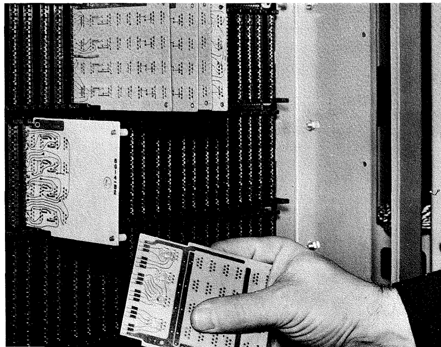
Fig. 4—Platter with connectors and plug-in card.
