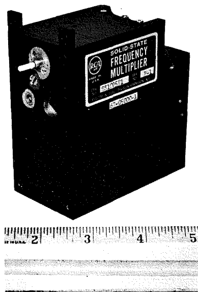
Fig. 3—Packaged ruggedized SS-1025-C-band harmonic generator.
