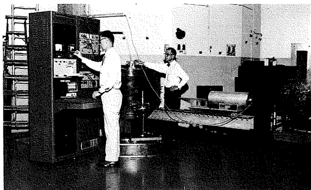
Fig. 8—D. A. Ross and J. G. White adjusting the neutron spectrometer built by RCA and installed at one of the beam ports penetrating the concrete pool wall.
