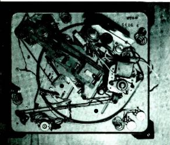
Fig. 5—Bottom view of 2-watt transistorized portable Victrola showing motorboard and mounting of components.
