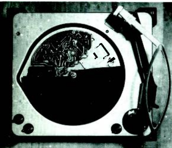
Fig. 4—Top view of the 2-watt stereo amplifier with turntable cut away to show printed circuitry.
