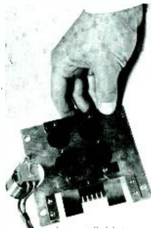
Fig. 2—Special fixture to hold targets in evaporator; four disks are silicon wafers; cylindrical device is film thickness monitor.
