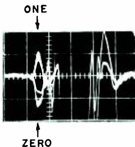
Fig. 16—Superimposed sense outputs from corresponding bit of eight words.
