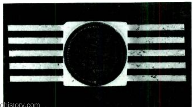
Fig. 5 — Welded 0.25" x 0.25" integrated-circuit packages.
