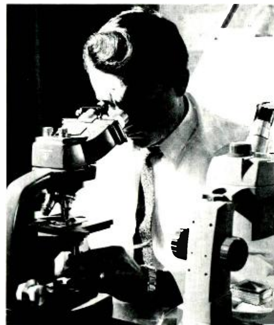
Fig. 12—High-power microscope used to observe edge definition in the photomasks.
