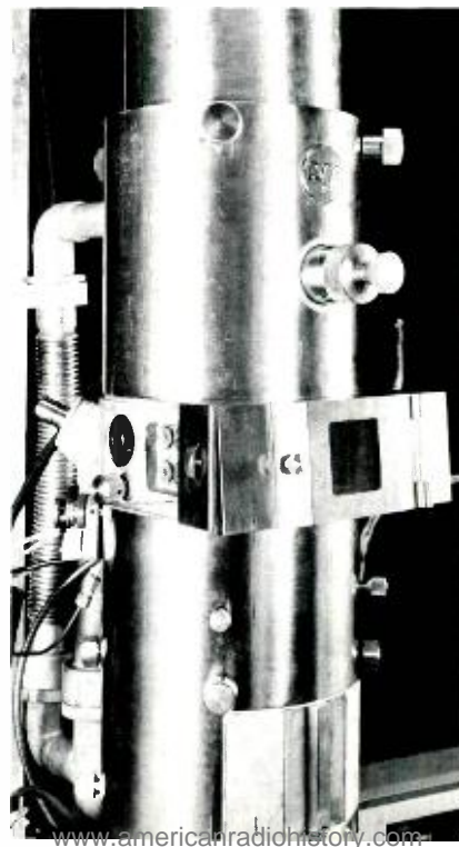
Fig. 3—Universal chamber showing specimen heater in place in the stage, cold baffle behind stage, and electrical feed-through in chamber wall.
