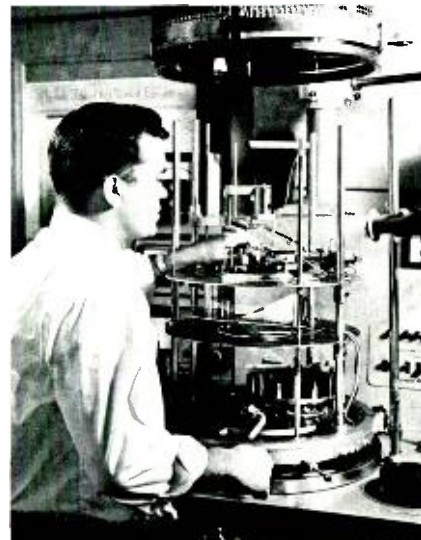
Fig. 14—H. P. Lambert mounting the jig for evaporation.
