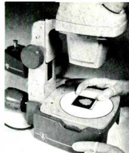
Fig. 11—Stereomicroscope used to detect surface imperfection in the photomasks.
