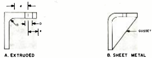
Fig. 7—Proper fitting design.
