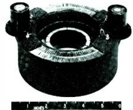
Fig. 8—Thermoelectric photocathode (TPC) cooler: This TPC is completely self-contained refrigeration machine. The thermoelectric material, the air heat exchanger, and the circulator fans are all contained in a package weighing only two pounds. The high performance, the proven reliability, and the practical power requirements (28 volts-dc, 2.5 amps) make the TPC a practical unit for Army field use.
