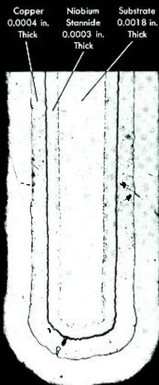
Fig. 1—Photomicrograph showing cross section of superconductive material.
