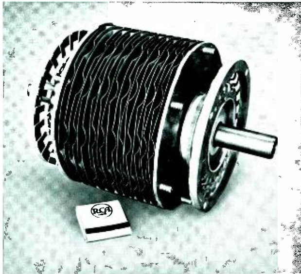
Fig. 6—Thermionic converter designed for operation in an external loop.
