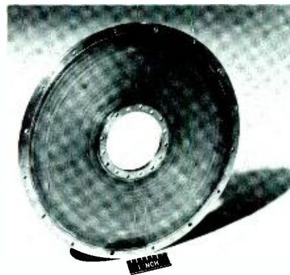
Fig. 7—Magnet module after plastic encapsulation to immobilize winding and increase strength.
