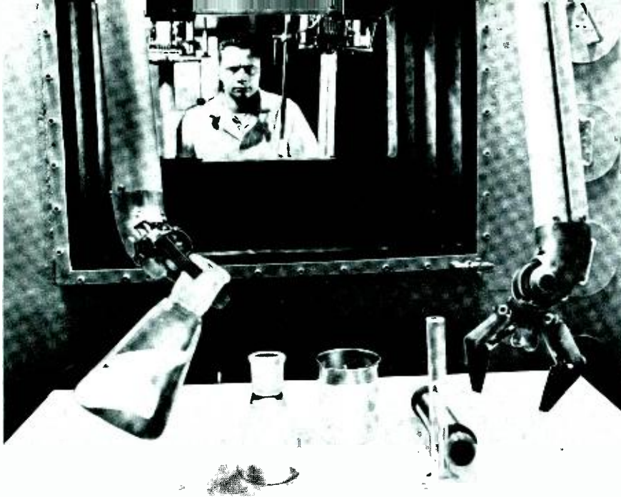
Fig. 1—Radiation hot cell for remote-controlled manipulation of high-level radiation sources. The window is 3 feet thick and is made of a radiation-resistant glass.
