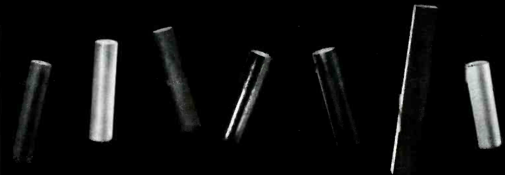
Fig. 1—Calcium fluoride standard laser rods (about actual size) cut from grown crystals.
