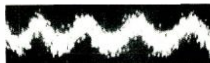
Fig. 2—Detection of an optical signal modulated at 200 Mc as displayed by a pulse sampling oscilloscope.
