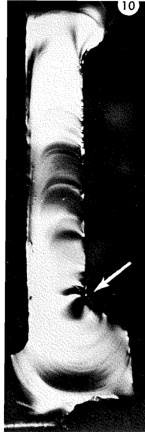
Fig. 10—Surface pattern of stem fracture which originated at metal particle indicated by arrow (10x).
