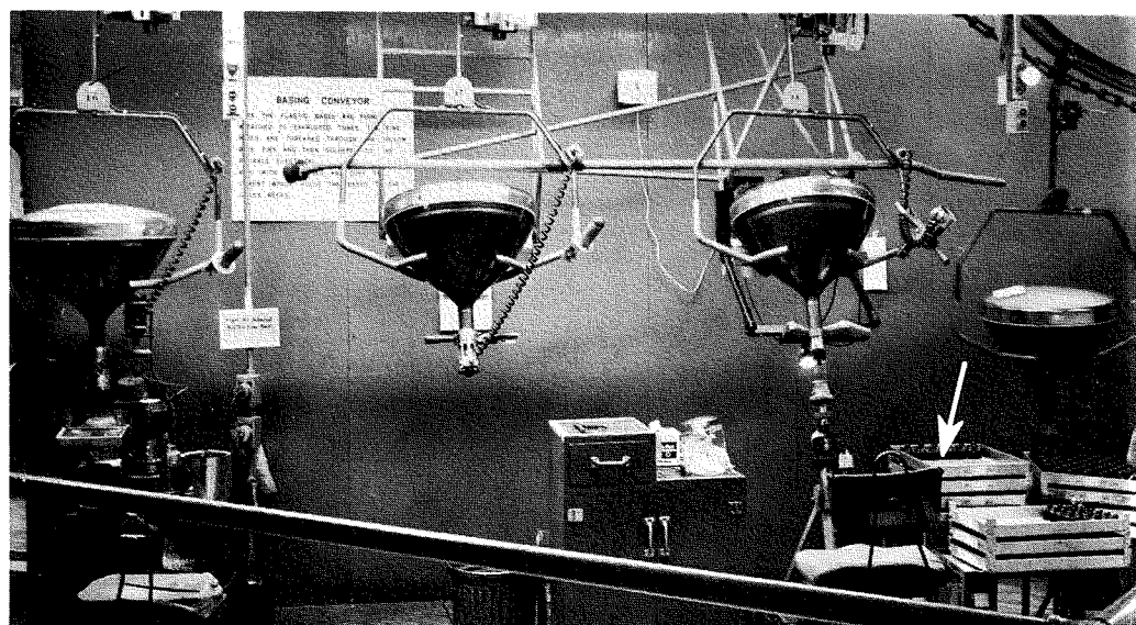
Fig. 9—Basing conveyor, where the plastic base (arrow) is attached to the exhausted tube. The wires are threaded through the hollow base pins by an operator at the right, and then soldered by another operator at the left.
