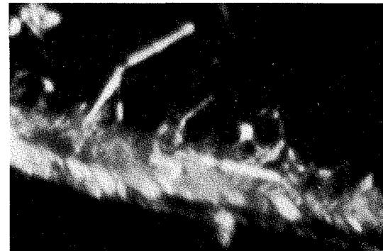
Fig. 7—Tin whiskers growing from an electro-plated tin film (200X).
