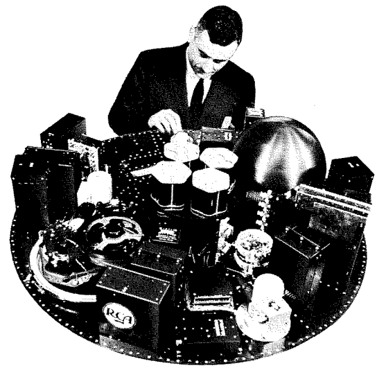
Fig. 6—Sidney Sternberg, Chief Engineer of AEP, inspecting the first assembly of a TIROS I satellite. This is not a flyable model, although identical in construction, because of the severe tests to which it was subjected.
