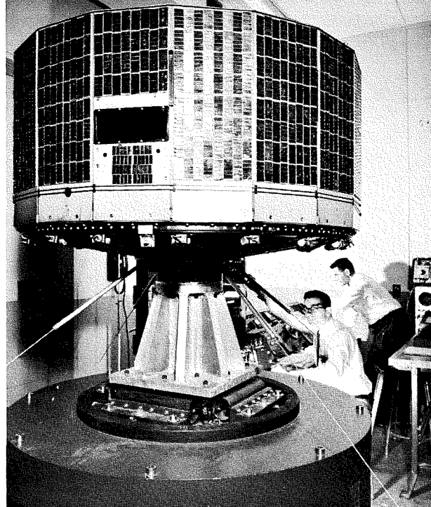
Fig. 10—The TIROS satellite on a vibration table at AEP, with G. Hieber at the controls and E. Grzegorzewski monitoring test readings.
