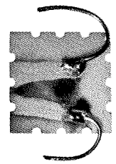
Fig. 4—Ultrasonically cleaned, silver-metalized wafer that withstood 50 volts d-c.
