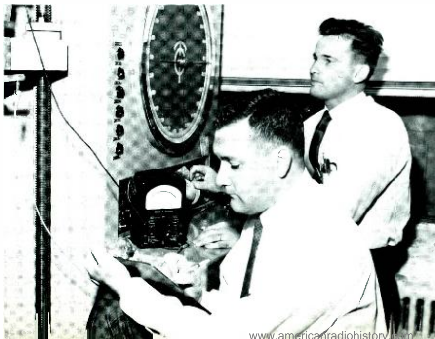
Fig. 2—The author, Dr. L. H. Cutler (foreground), and a laboratory technician, R. J. Forster, measuring changes in conductivity of a conductive adhesive as tensile stress is varied.
