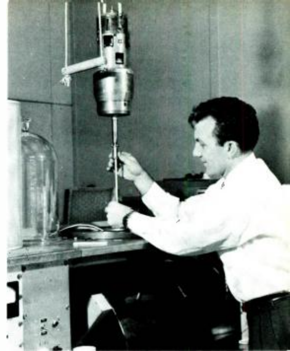
L. A. Zanani changing ferrite samples on a magnetometer, which measures the magnetic movement of materials.
