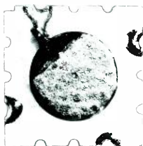
Fig. 2—Dry electrolytic capacitor in microelement form (rated up to 60 \mu f-volts). The tantalum anode measures approximately 0.180 inch diameter and can be made from tantalum in various forms. Tantalum surface is oxidized to provide dielectric coating. A metallic cathode layer is applied by silk screening. Additional materials are used in making connections and terminations.
