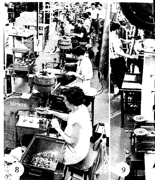
Fig. 8—These spinning machines are forming stereo record-changer parts. The machine rollers are activated by a foot lever to form round heads on the rivets of fastened parts.
