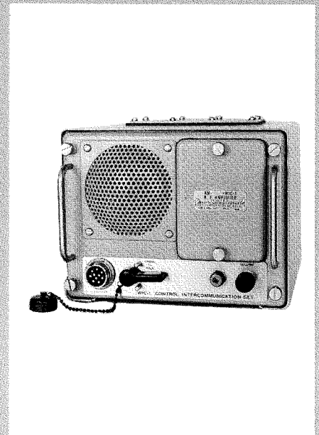
Fig. 6—Control unit of submarine Intercommunication Set AN/WIC-1. This unit contains a one-watt amplifier and a loudspeaker which is also used as a microphone.
