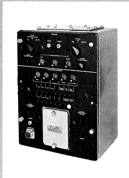
Fig. 5—Periscope station of submarine Intercommunication Set AN/WIC-1. The control unit of Fig. 6 is also associated with this unit.
