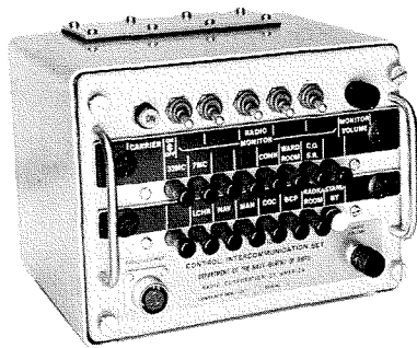
Fig. 7—Control unit for the submarine's missile control center. This is a part of the submarine Intercommunication Set AN/WIC-1.
