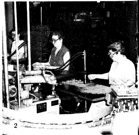
Fig. 2—A view of a conveyerized high-production resistance-welding line where each of four machine operators weld four to seven items to a 4-speed stereo record changer motorboard.
