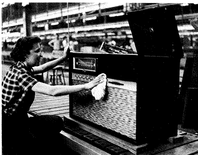
Fig. 7—A finishing and polishing operation is being performed on a SHC-6 "Victrola" console prior to packing the instrument for shipment. All large consoles are assembled by use of the slat-line conveyor shown here.
