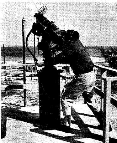
The tracking telescope, such as this one shown in operation at Eleuthera AAFB, is one of many optical systems used in missile tracking.
