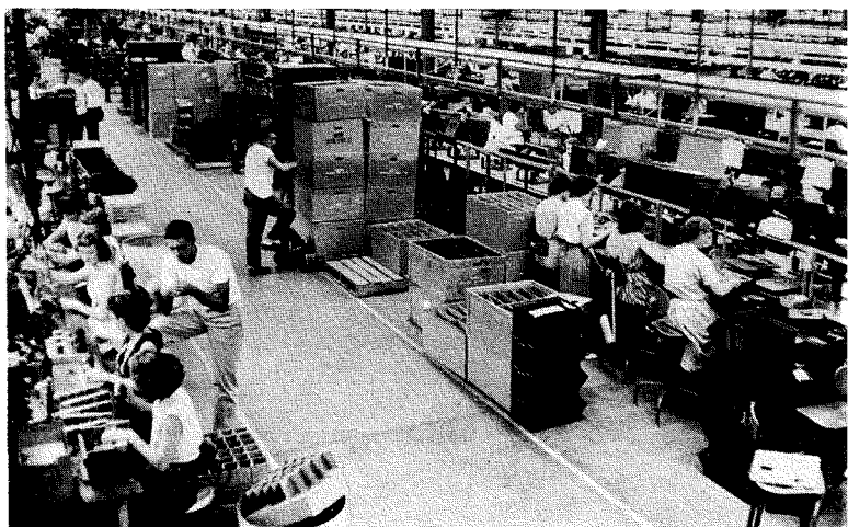
An overall view of the record-changer and amplifier assembly lines at RCA Victor's factory at Cambridge, Ohio. The plant, world's largest producer of packaged hi-fi instruments, has fifteen assembly lines capable of turning out 6,000 sets in an eight-hour shift. Inset is one of the instruments in RCA's complete hi-fi line.
