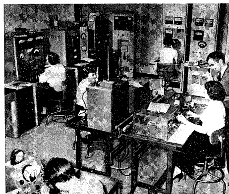
Fig. 6—S. C. Simons of Test Engineering checks life testing of transistors in Testing Laboratory. Life tests and design checks on both factory product and engineering samples are made by this group.
