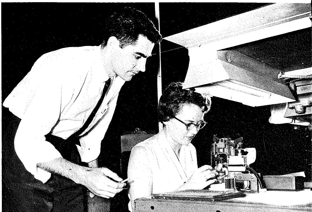
Fig. 5—Manufacturing engineer William Dibble is observing Marge Grubel as she inserts and welds the heater on a 117Z3 mount assembly.
