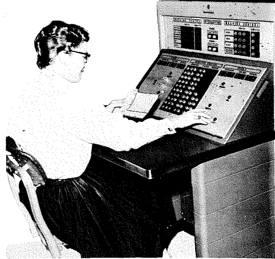
Fig. 7—System Operator Console—The System Operator directs the operation of the system from this console. She determines which operations to initiate, dispatches machine set-up tasks to the other members of the operating team and controls the operation of the machines in the system.
