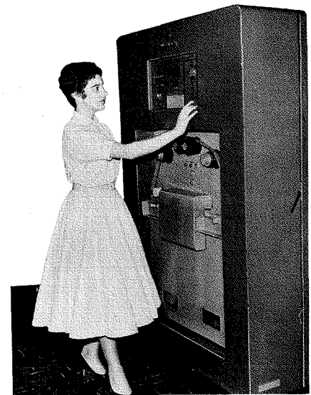
Fig. 5—Paper Tape Transcriber—The control panel for the Paper Tape Transcriber has been located at "eye" height for easy viewing, and all the controls for operating the machine are easily accessible to the operator.
