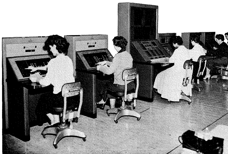
Fig. 6—System Central Control Room—The control room is completely enclosed to provide a quiet working environment for the operators and air conditioned for comfort. Close attention was paid to proper lighting and the choice of colors to make the room pleasant to work in and the consoles faces easy to read. The operator consoles are located on the right and the two corresponding verifier consoles on the far left. The Monitor Console is the large console in the center and the System Operator Console is located to the right of the Monitor. All the consoles were designed for optimum operator comfort in working with the controls and indicators.
