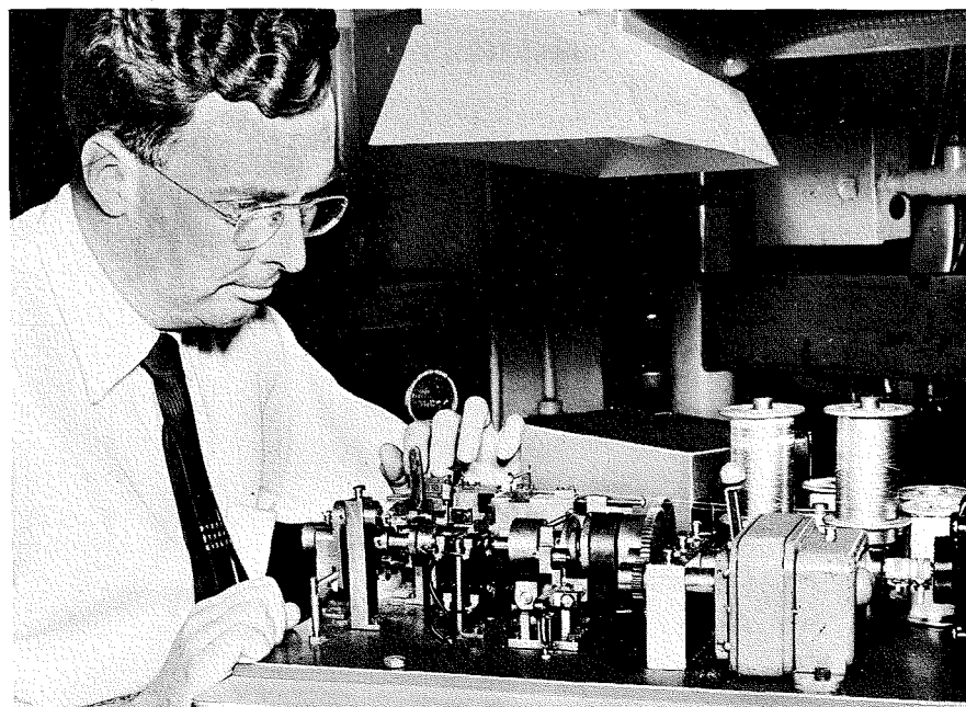
Fig. 8—Equipment Development engineer George Shaffer testing an automatic cathode-tab feeding-and-welding machine in the Equipment Development Shop.
