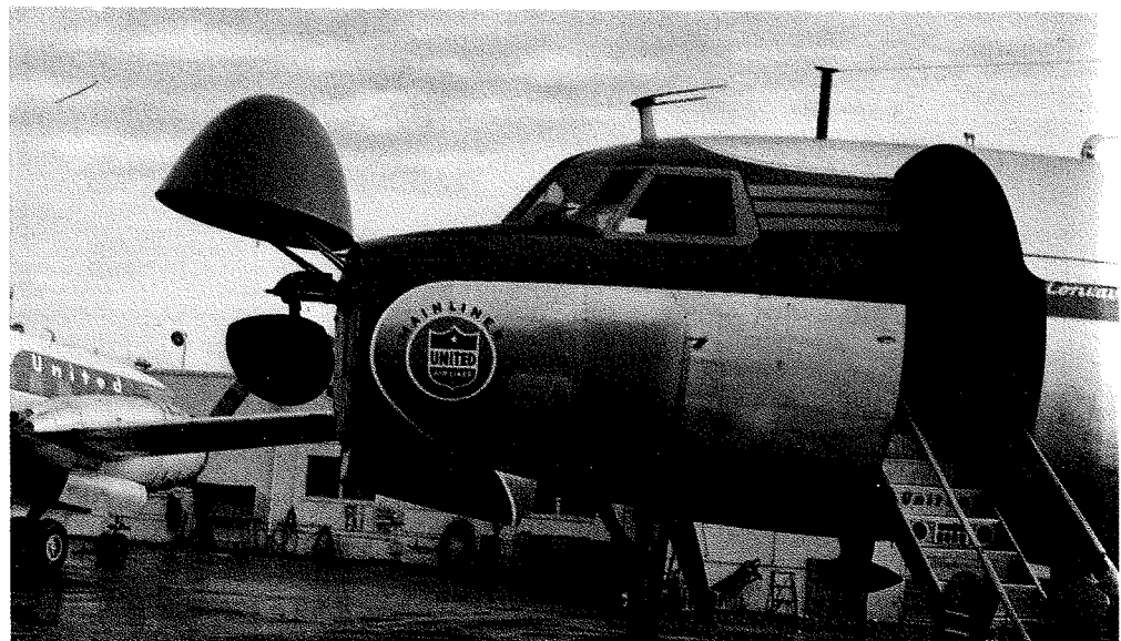
Fig. 11—Typical AVQ-10 Antenna Installation, Convair 340.
