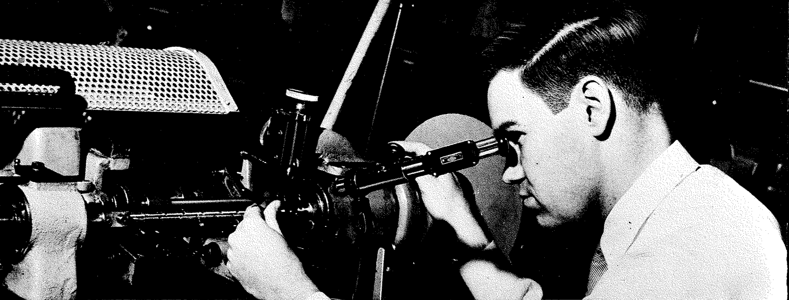
Fig. 4—Development Engineer, D. B. Pearson is shown inspecting wire-feed mechanism on RCA grid Lathe.
