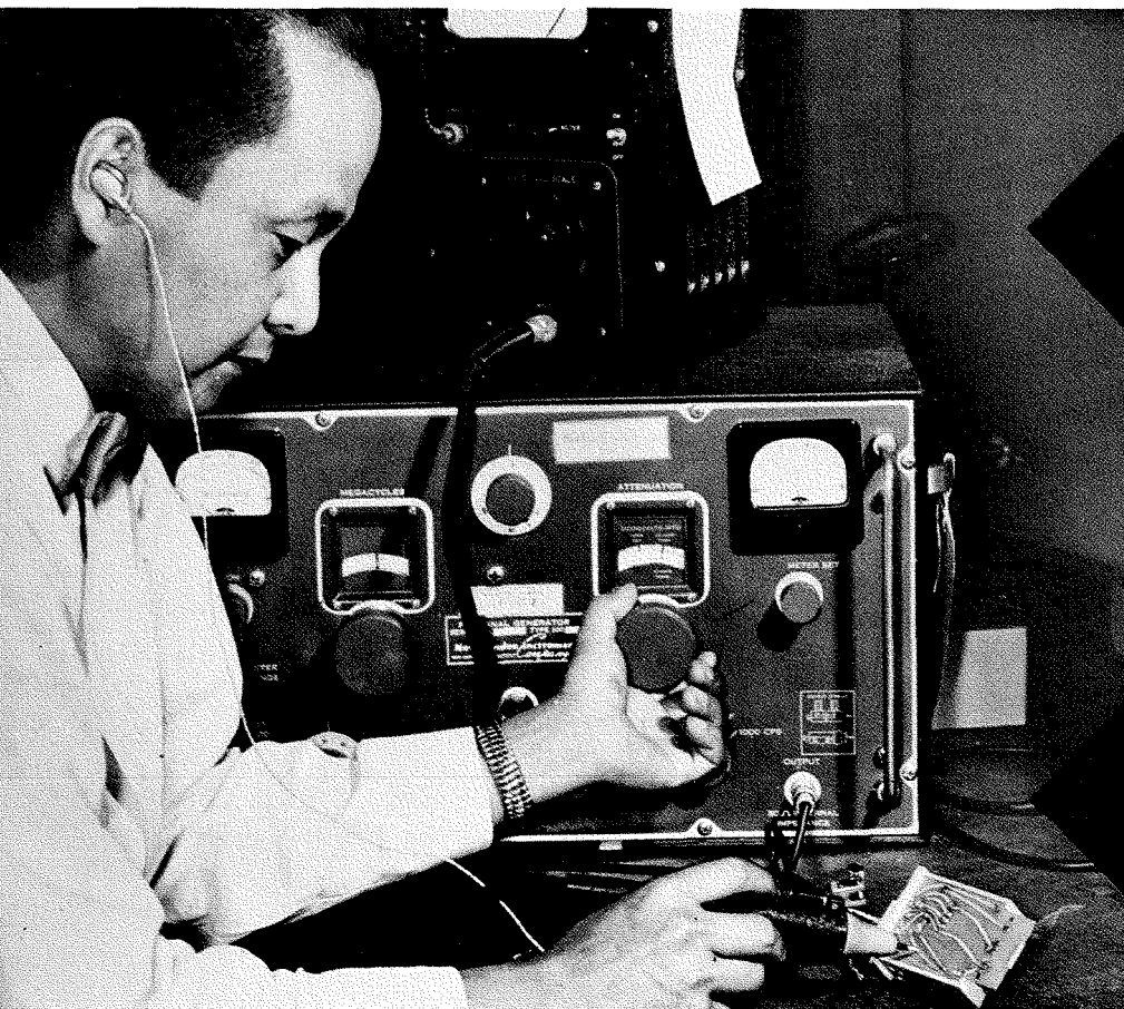
Sadao Okafuji, Surface Communication Engineer shown performing a test on a complete ultra-miniature, transistorized F-M radio receiver which utilizes modularized construction. Note the size relationship of test probe and receiver.
