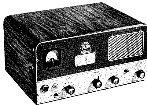
GOLDEN HERALD (MODEL ET-8057) —100 watt plate input, 50 watt antenna power transmitter with eight crystal controlled channels in the 2-3 Mc band. Receiver has eight crystal controlled channels. A press-to-talk "Mike" or optional handset may be used. Golden anodized front panel with simulated mahogany finish metal cabinet. Designed for larger cruisers and yachts having 12, 32, 115 volts DC or 115 volts AC power supply. Typical salt water ranges 50 to 100 miles. Price $615.00.
