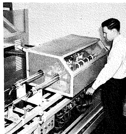
Fig. 3—D. B. Pearson is shown making adjustments on the RF Zone Purifier which produces germanium of high purity by passing successive molten zones through an ingot.
