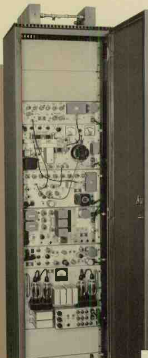
Fig. 2A—Cabinet-mounted 2000-mc terminal, without standby equipment.
