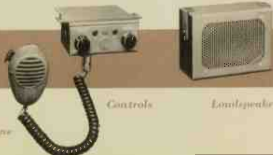
Fig. 3—RCA mobile radio. Transmitter-receiver mounts in car trunk or truck cab. Speaker and controls mount under dashboard.
