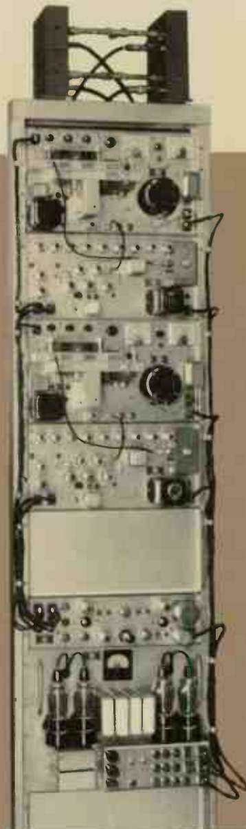
Fig. 3A—Rack-mounted 2000-mc drop-channel repeater, without standby.
