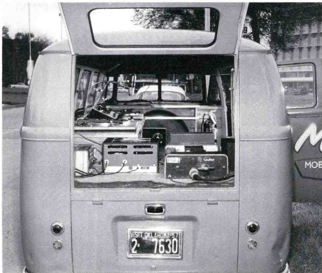
FIG. 2. Rear view of KRMG Mobile Studio. Note two-way radio "Carlone" unit at right.
