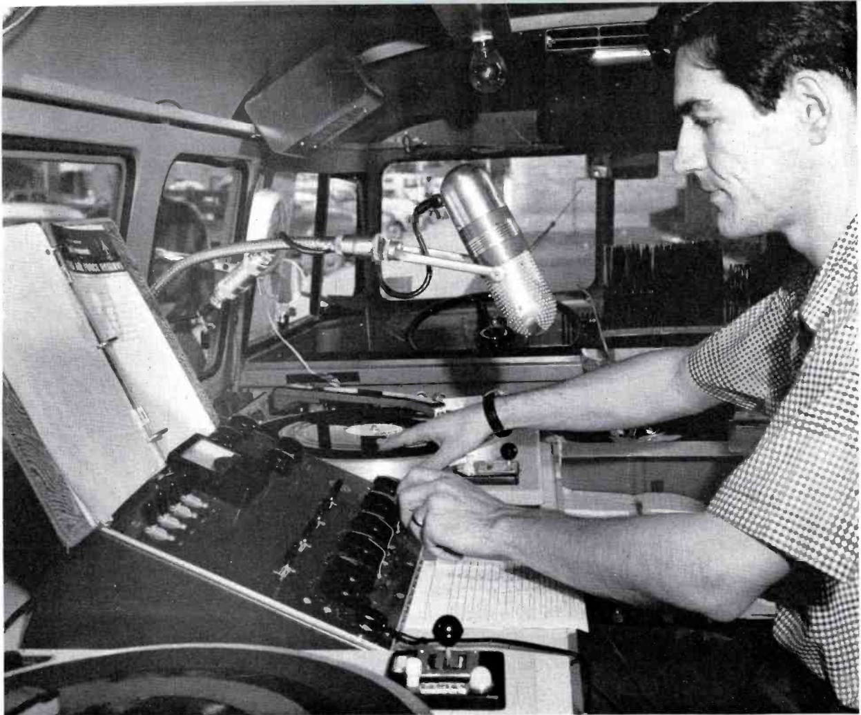
FIG. 3. Complete D-J studio is built into KRMG mobile unit using Type BC-5A Audio Consolette. There is sufficient room for convenient operation.
