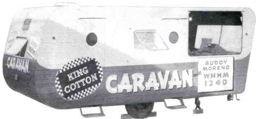
FIG. 21. This is a typical mobile studio of the type employed for remote broadcasting. (Shown here is the WHHM mobile unit with BC-5A audio-console inside.)
