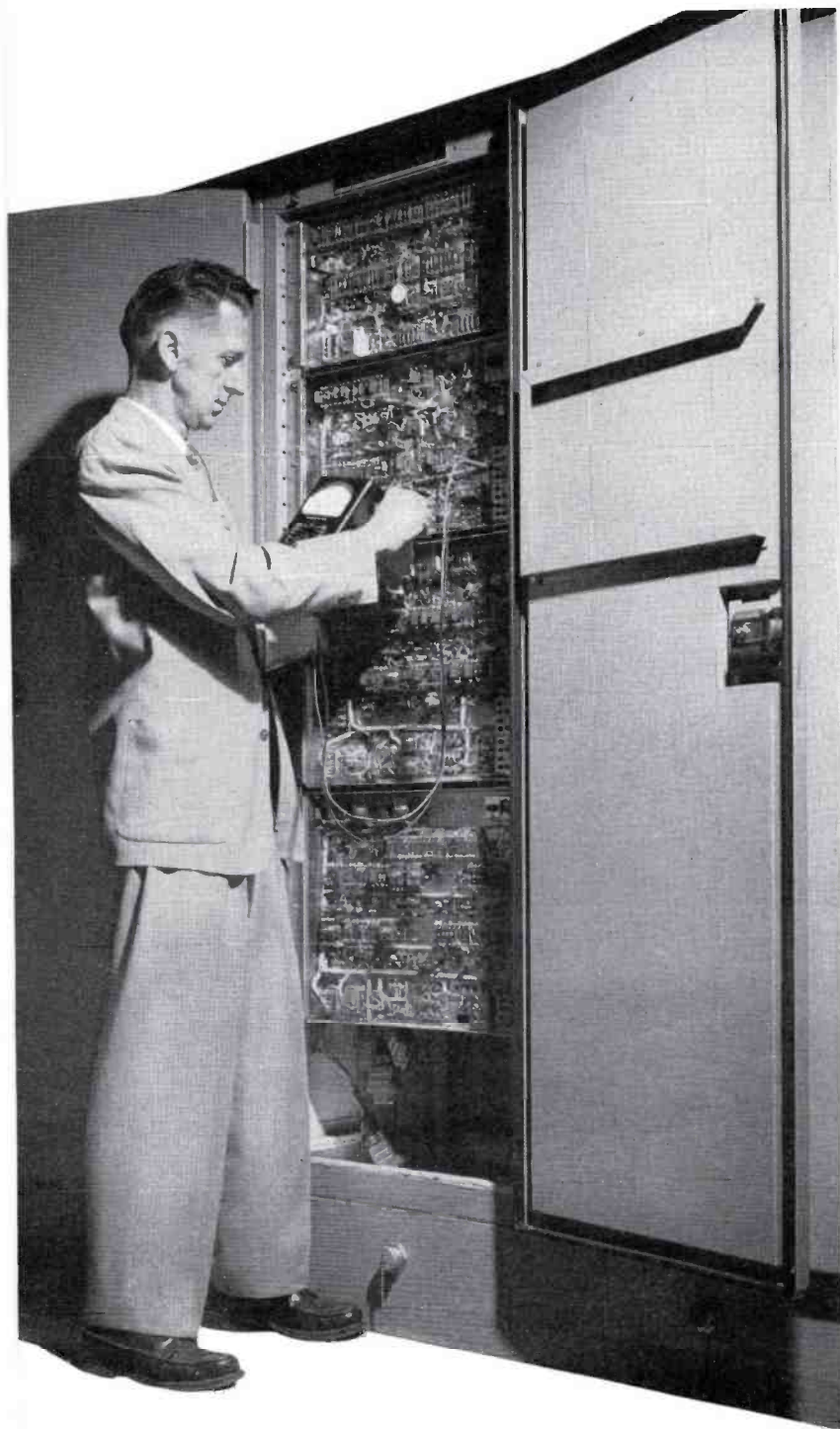
FIG. 4. Merritt Sheeder, Project Engineer, is making a circuit check at the readily accessible underside of an Instrumentation Radar Chassis.
