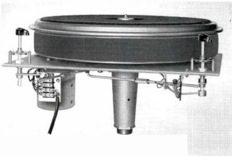
FIG. 3. The 16-inch turntable platter is made of a sturdy 14-lb aluminum casting. Rumble is eliminated by mounting the drive motor on a separate plate and supporting it by vibration mounts. All posts and shafts which provide bearings for cams and arms are assembled to a common plate to insure proper alignment.
