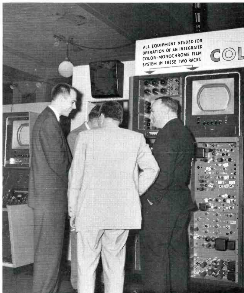
FIG. 8. Complete auxiliary equipment for RCA color-monochrome film system is housed in two cabinet racks.
