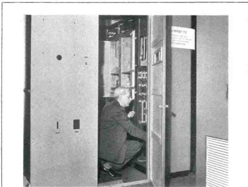
FIG. 17. Walk-in construction offers easy inspection and maintenance of TT-6AL.
