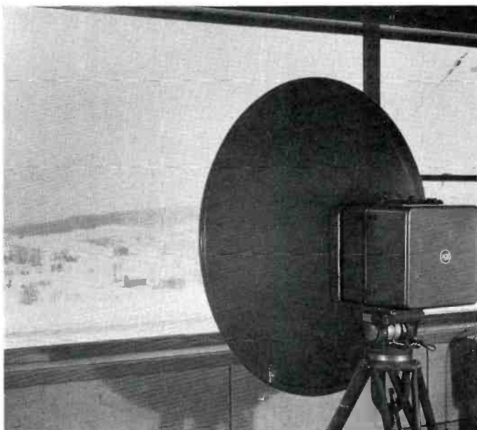
FIG. 9. Spare microwave receiver is mounted in the main transmitter room—conventional tripod allows movement for remote pickups.
