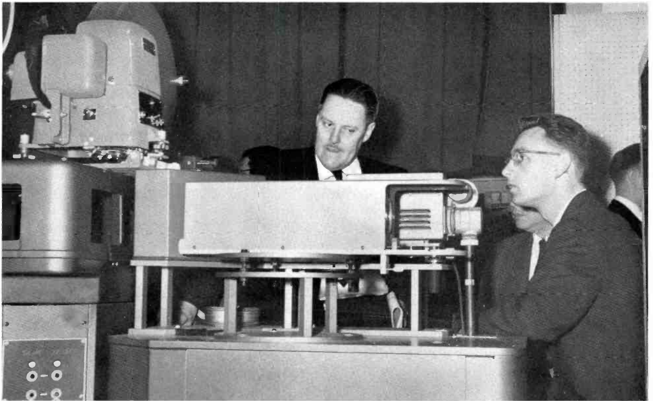
FIG. 5. Simple extension lens system adapts RCA 3-V color film system for opaques and live action.
