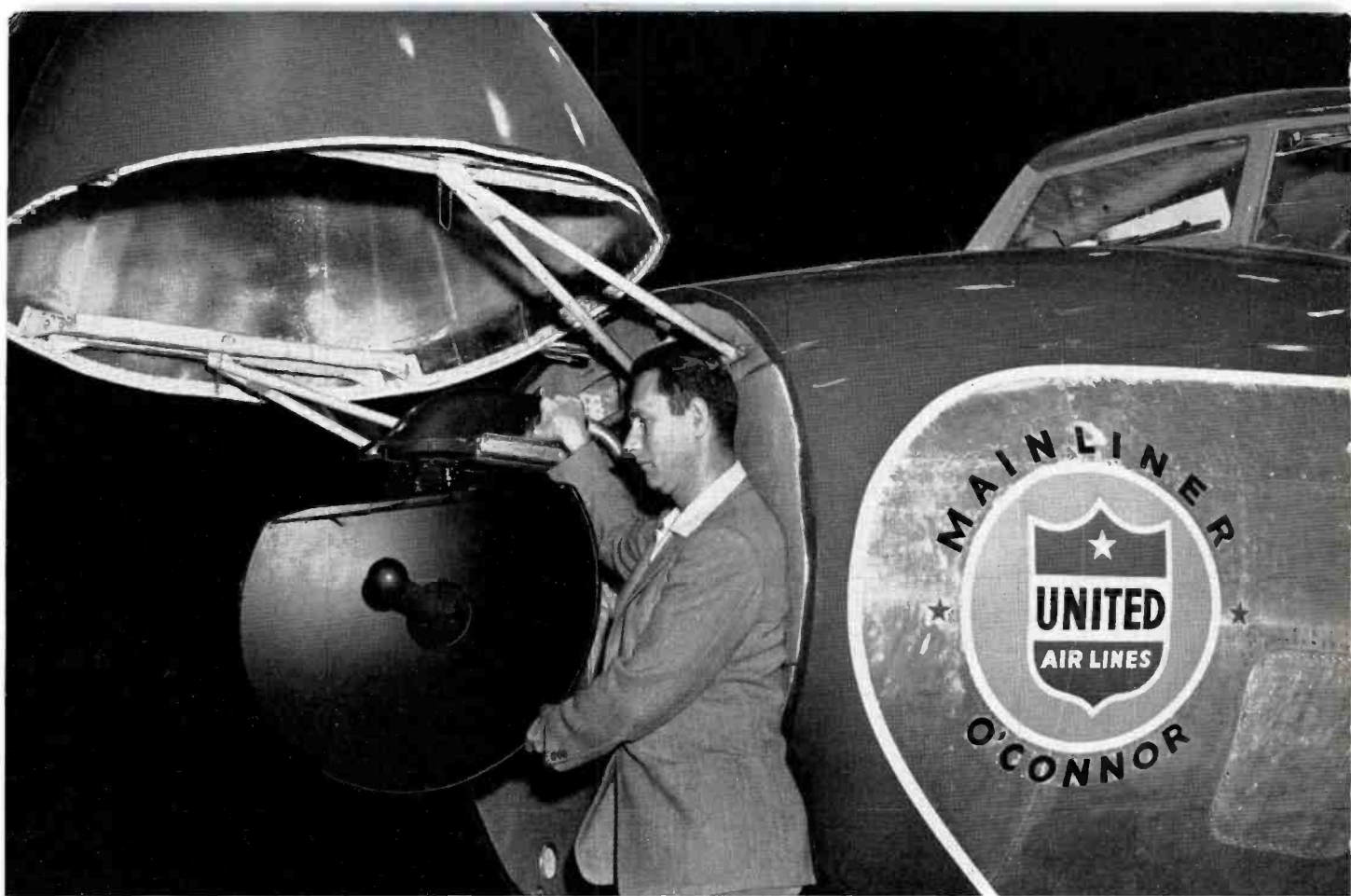
L. E. Sebald, project engineer at the San Francisco maintenance base of United Air Lines, demonstrates antenna of RCA C-band radar on "Mainliner O'Connor." It is the first installation in a $4,000,000 program to equip the company's entire fleet with the new weather-mapping device. Nose of the Convair 340 has been extended 28½ inches to house radar antenna and gear mechanism.
