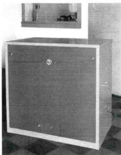
FIG. 2. External view of Automatic Turntable. Note front panel locks at upper corners. Cable access parts at bottom.
