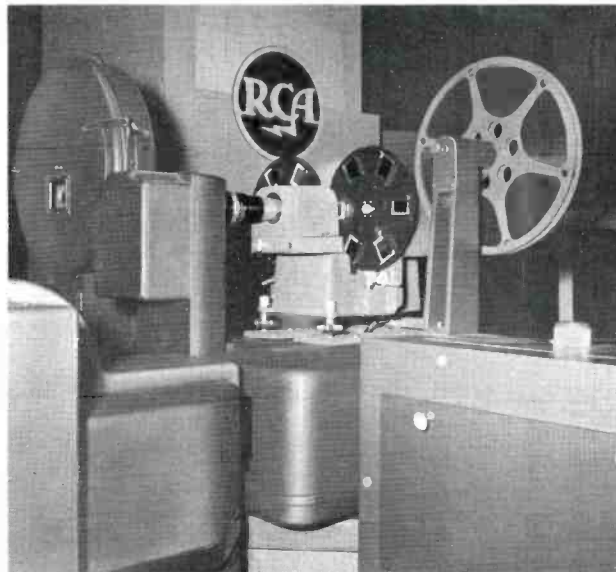
FIG. 7. New periscope attachment offers fourth input to the TP-15 Universal Multiplexer.
