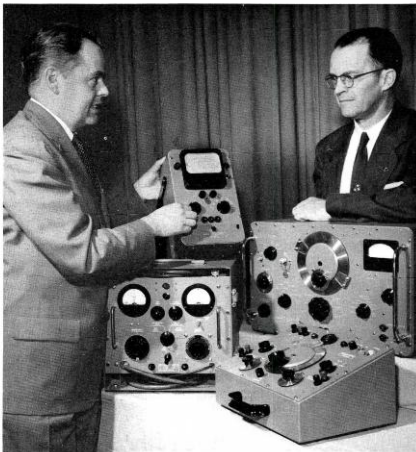
Dr. James Hillier (left), Chief Engineer, RCA Commercial Electronic Products, discusses operation of vacuum tube voltmeter with C. O. Caulton, Manager, New Products Administration. Other instruments shown include r-f power meter, left; signal generator, right background; and impedance bridge, right foreground.
