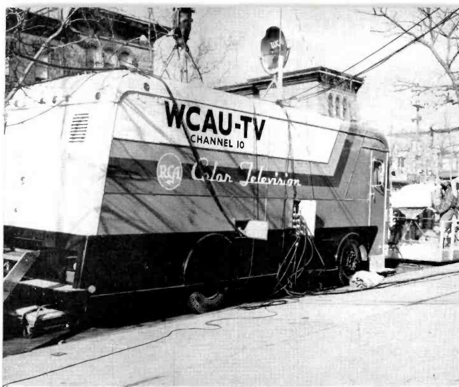
FIG. 5. On this side of the color mobile unit, the receptacle at the right contains sockets for connecting audio, video, telco lines and microwave facilities. At the left is the power-line receptacle.
