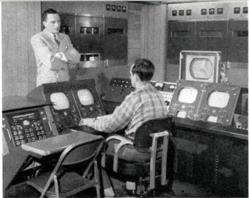
FIG. 23. Control console for 3-V film system is in transmitter room.
