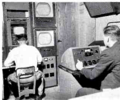
FIG. 2. Control room section of truck—showing camera controls (left) and audio control (right).
