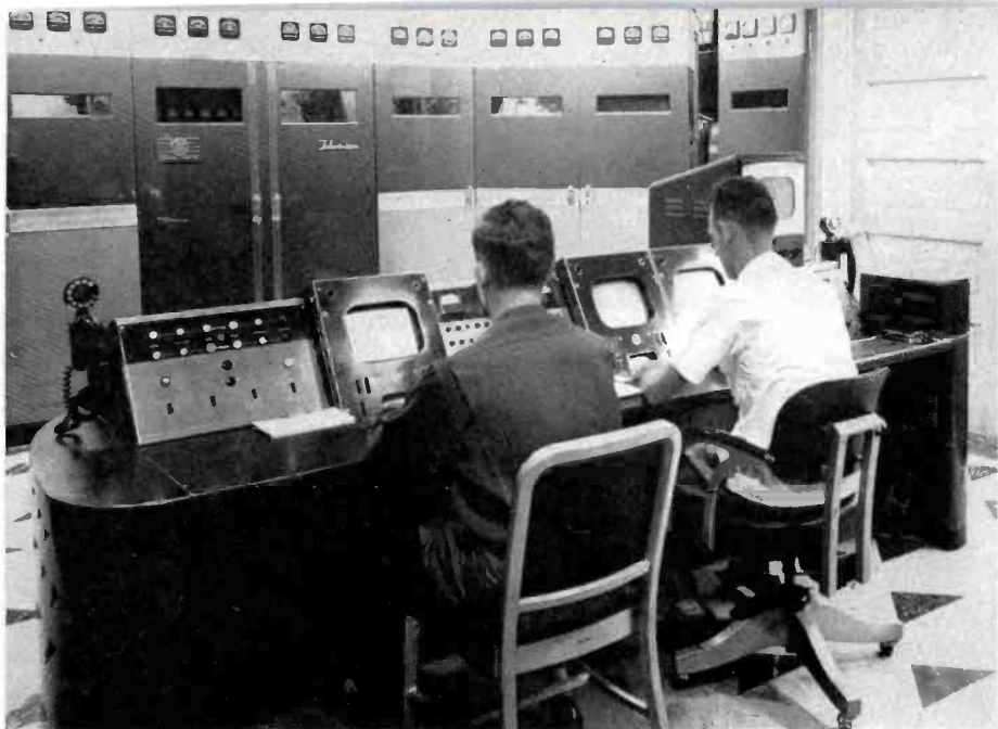
FIG. 24. KMTV uses an RCA TT-5A 5-kw VHF transmitter with a TT-25AL amplifier.
