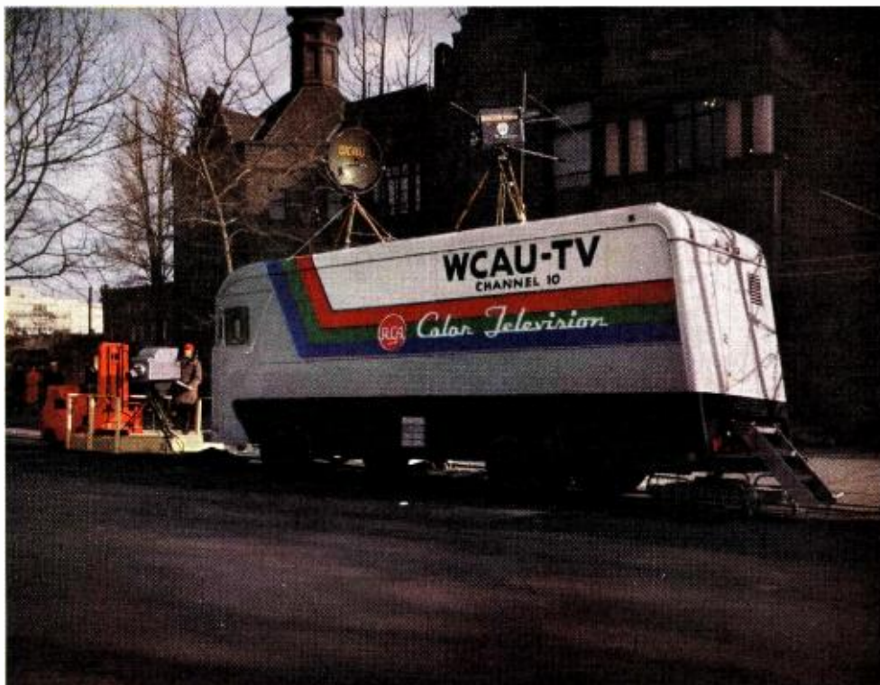
FIG. 4. On the day before the parade this color mobile truck was in place at the South Broad Street location. In front of the truck, one of the TK-41 live color cameras is mounted on the specially designed wooden platform. Good maneuverability was obtained by the use of these fork-lift trucks for the color cameras.
