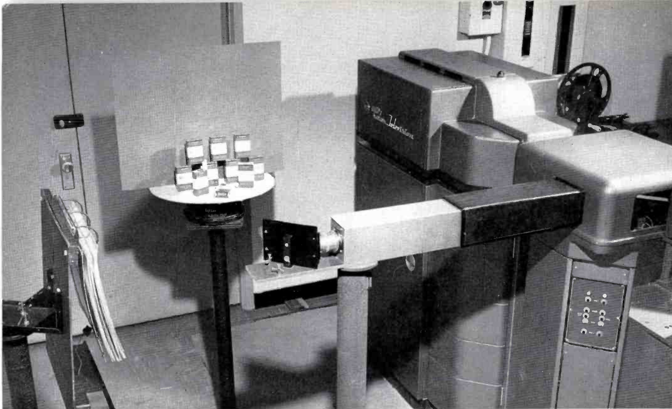
FIG. 1. Lens system added to RCA TK-26A 3-V Color Film Chain for pickup of live color commercials and color opaques.
