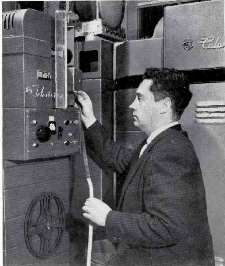
FIG. 3. Merle Severn prepares to preview color film he shot for Channel 4's news program "Deadline!" and developed in 90 minutes. Fast-processing technique makes possible local news coverage in color the day it happens. Development means television can now do substantially everything in color that up to now has been possible only in black and white.
