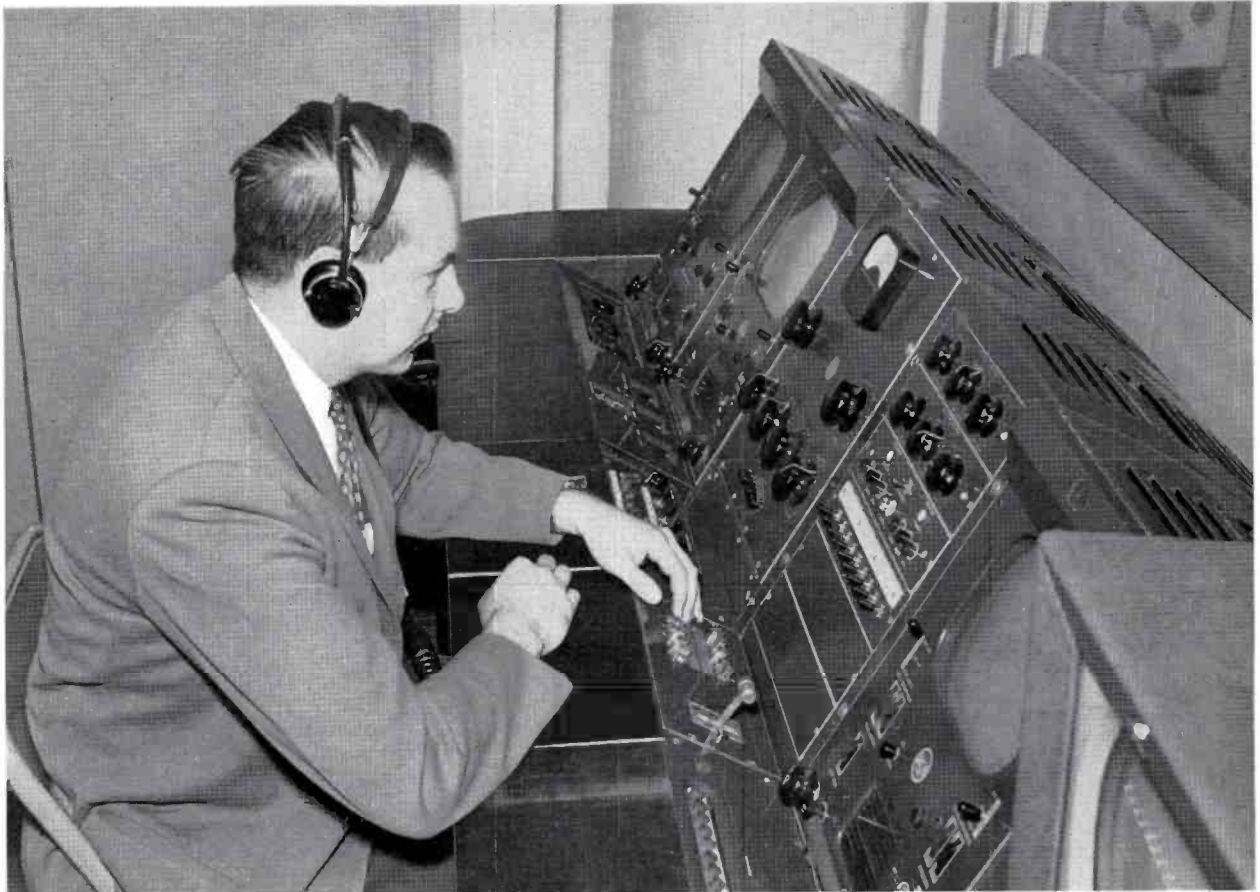
FIG. 1. A typical arrangement showing the TS-5A Video Switcher supplementing the facilities of the TC-4A Audio/Video Switching Console.
