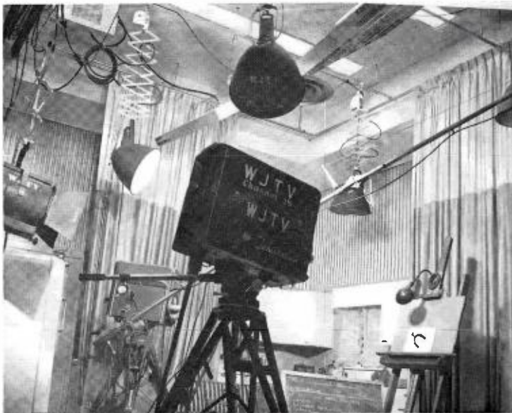
FIG. 5. View of a corner of the WJTV studio which shows a typical lighting and camera arrangement.
