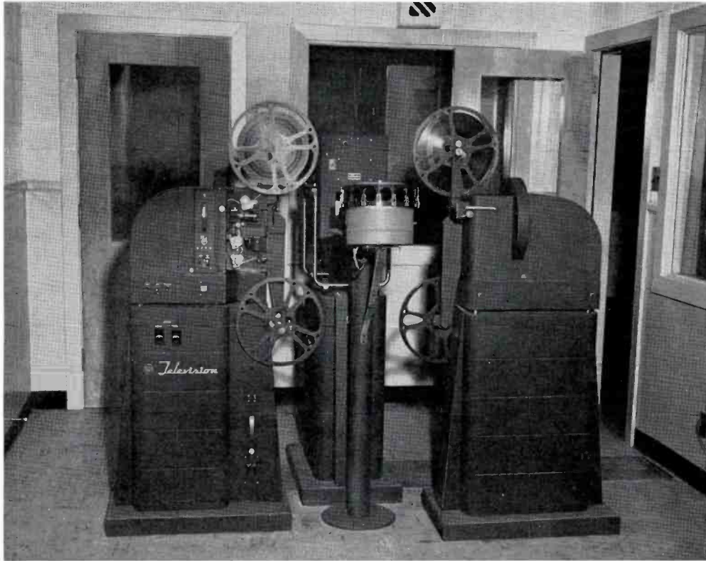
FIG. 7. View of the WJTV film projection room showing the use of RCA 16mm projectors, TK-20 film camera, and automatic slide projector.
