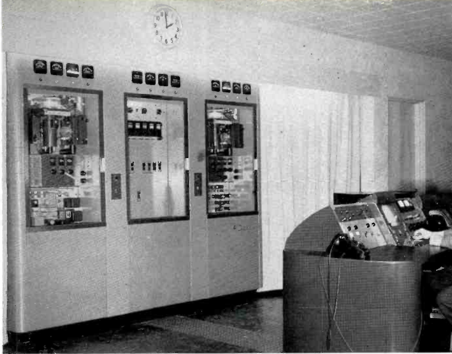
FIG. 2. WHP-TV's Chief Engineer, Dan Leibensperger, is shown at transmitter controls. Transmitter is the RCA TTU-1B.
