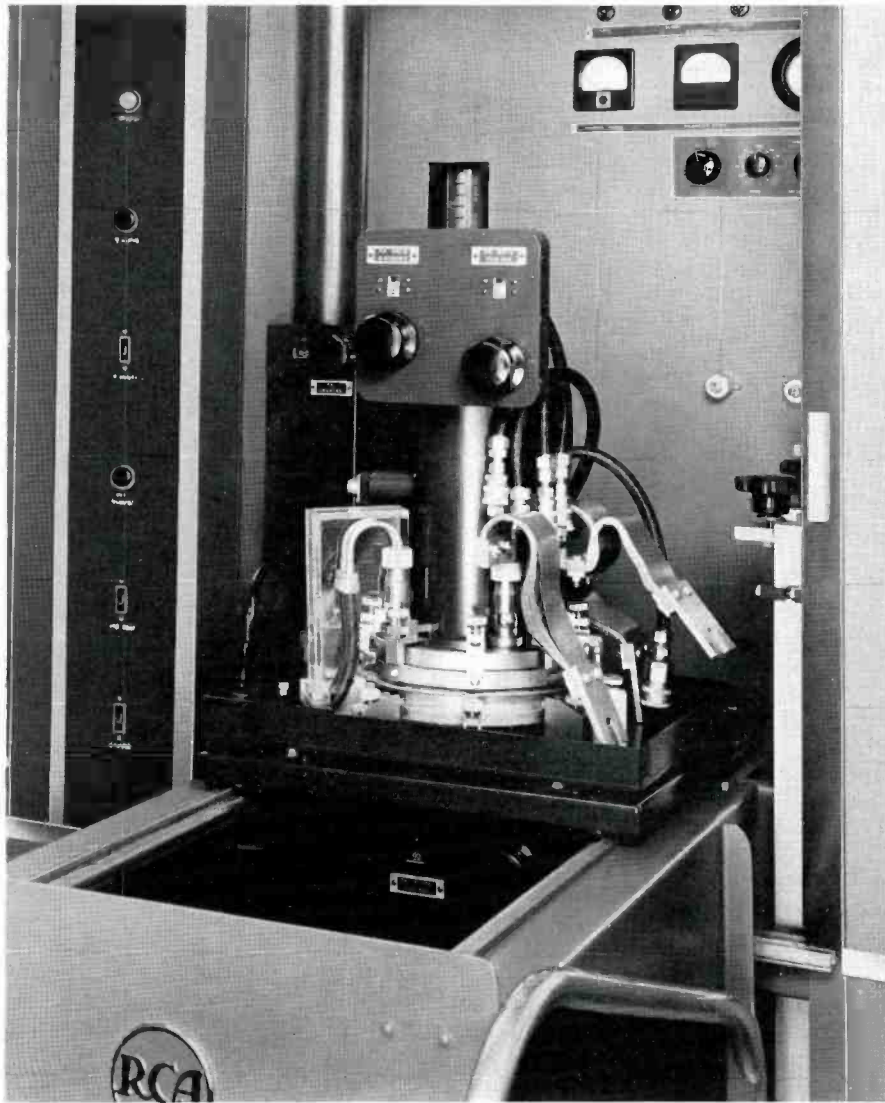
FIG. 5. A spare "P.A." cavity, supplied as a part of the transmitter, simply glides from a dolly into proper position in the P.A. cabinet. Compactness of the tetrode and unique cavity construction permits the operator, unassisted, to replace the complete final stage with an auxiliary amplifier within five minutes.
