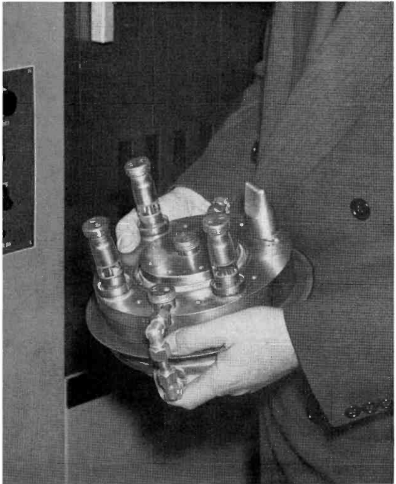
FIG. 4. Closeup view of the new small-size, RCA 6448 used in the TTU-12A Transmitter. The same conventional tube (RCA Type 6448) is used in the Aural and Visual "P.A." Use of conventional types of tubes throughout results in economical operation, easy maintenance, and simple, straightforward circuitry.
