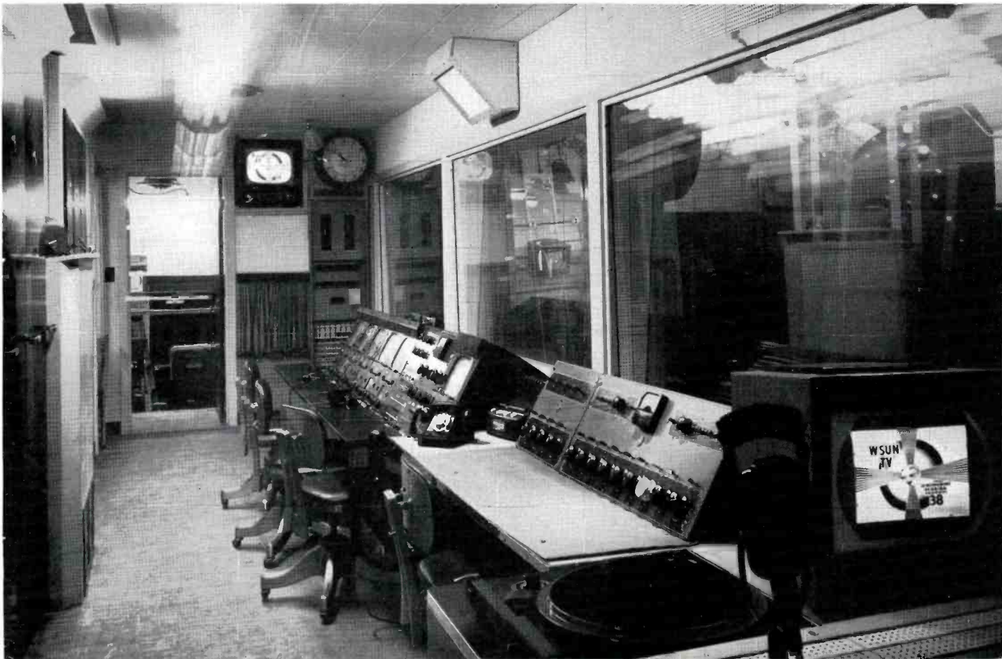
FIG. 12. Studio Control Room. From far end, console equipment consists of two monitors for studio cameras, two film camera monitors with control units, a line monitor with TS-10A switcher, two console housings comprising the TC-4A switchers and a preview monitor. Moving forward from the telephone and intercom unit is the BCM-1A audio mixer and the BC-2B audio console. An RCA utility monitor and 70-D transcription turntable are in the foreground. To the left is studio rack equipment and the director's box. In the background is the film room and the studio lighting control panel.
