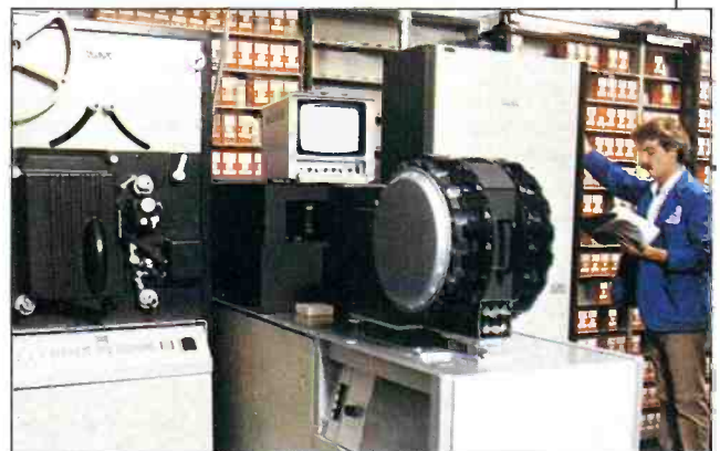
VTR operator in background checks out cart for commercial play. TK-29B Telecine System in foreground.
