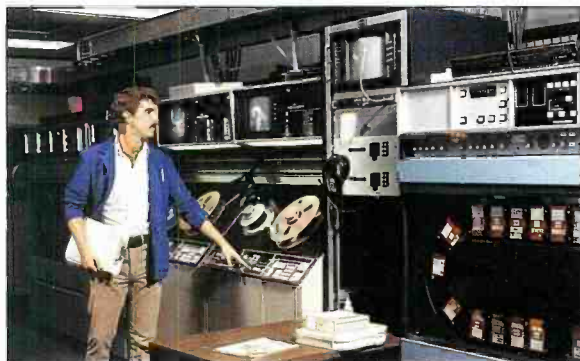
Tape center includes two Quad and two Cart recorders.
