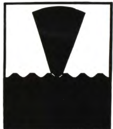
Needle B after playing a 16-inch record. (The shoulders on both sides wearing on the walls.)
