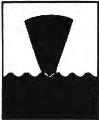
Needle C after playing a 16-inch record. (Emphasized shoulders wearing on both walls.)
