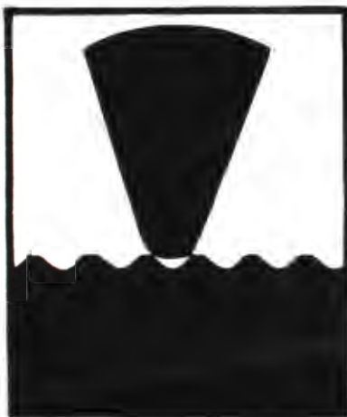
Needle C in standard groove before playing. (Note that needle rides the walls.)
