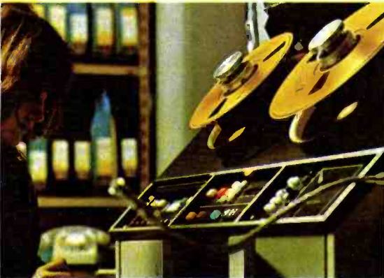
The new tape facility utilizes a TR-600 recorder for masters in the production of training courses eventually dubbed to cassettes.
