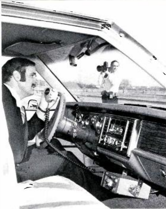
For greater coverage and communications versatility, TACTEC portable can also be used as a mobile radio with the addition of a vehicular charger and power booster.
