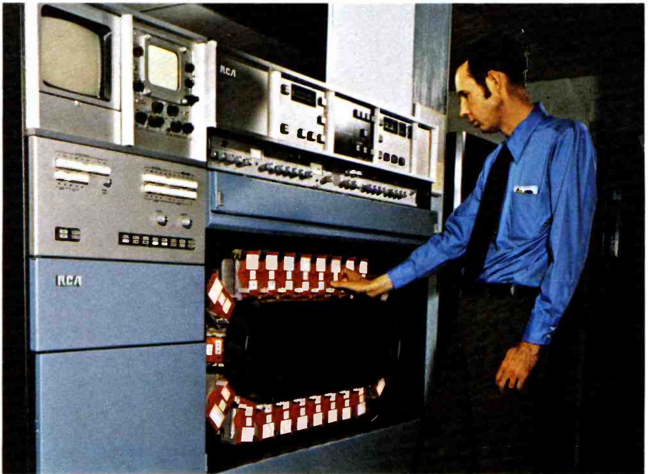
WFMY-TV Technician Jack Merritt gets station's TCR-100 ready for the day's action.
