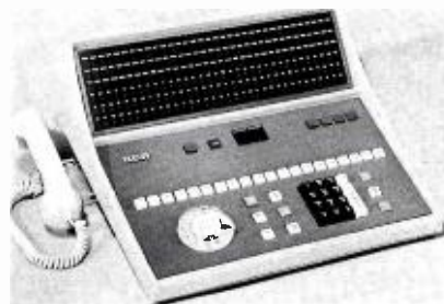
New electronic PABX system developed by RCA makes extensive use of LSI's for smaller size and increased reliability.
