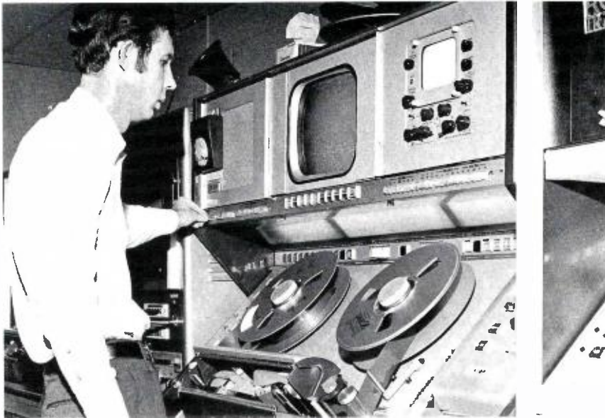
Addition of TCR-100 permits WFMY-TV to use TR-70 and other tape machines for production.
