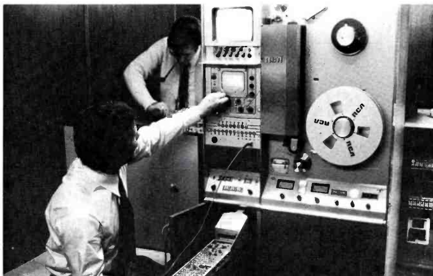
Inside Westward's remote unit, an engineer pulls a routine test on the newly added TR-60A VTR. The van is used to cover community events and produce on-site commercials for local businesses.
