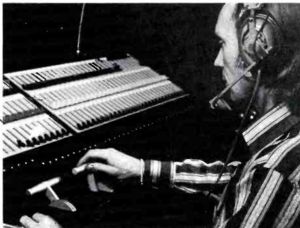
Time-saving remote dimmer lighting console features a 5-scene pre-set capability.
