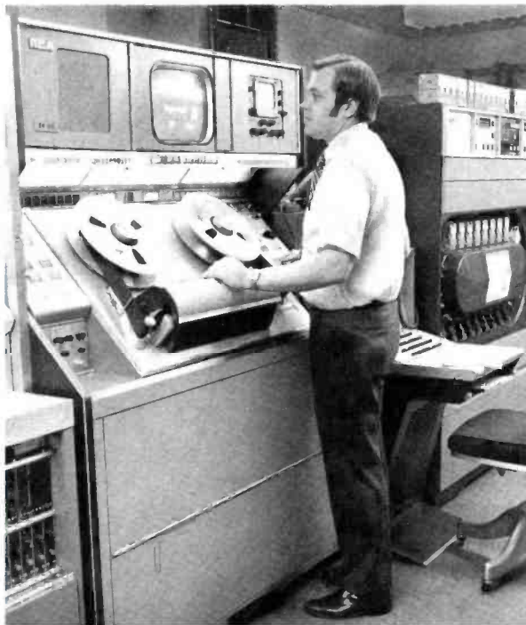
With the TCR-100 handling station breaks, more TR-70 operating time can be dedicated to production assignments.
