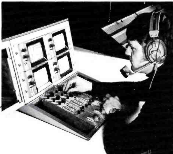
Joystick controls for TK-44 cameras are now located in the production area rather than in Master Control.
