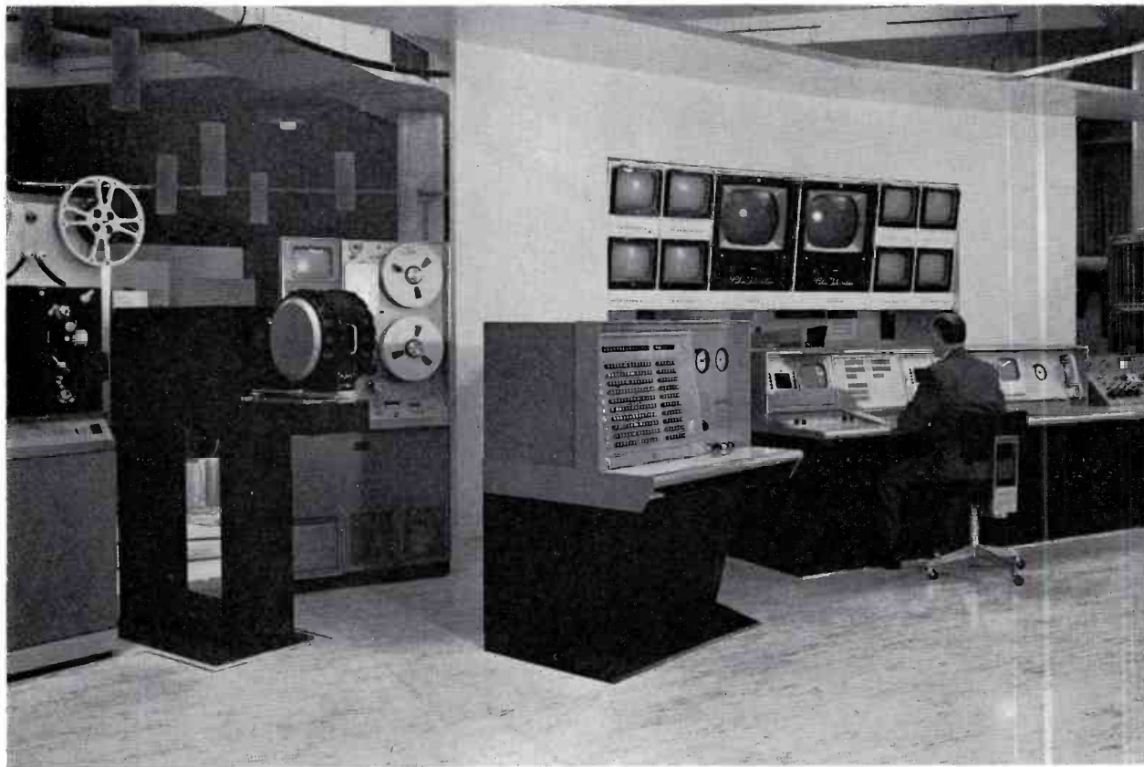
ONE OPERATOR CONTROLS EVERYTHING in this New Look conception of how a control room should operate. Revolutionary concept envisions video controls and machine operations combined with switching functions in a control central. The transmitter panel may also be incorporated into this master control console.
