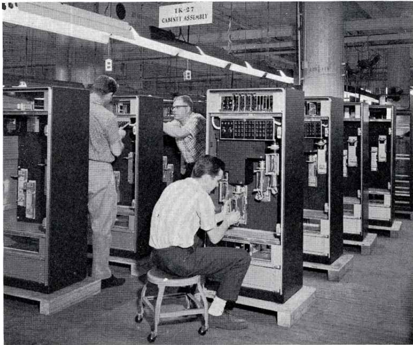
The four-tube system that distinguishes RCA's new TK-27 color film camera shows clearly in this view of cabinet assembly operations at the RCA Camden plant. Demand is heavy for all color equipment items.
