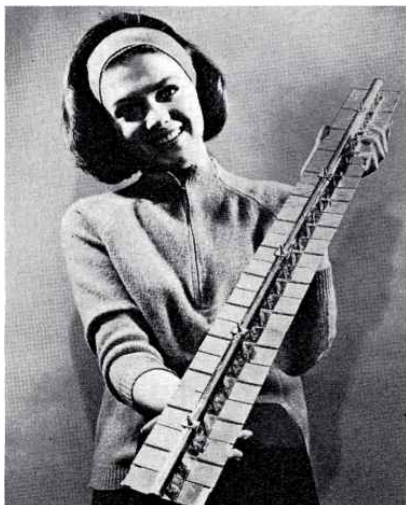
One of SNAP-10A's 120 thermoelectric modules.
