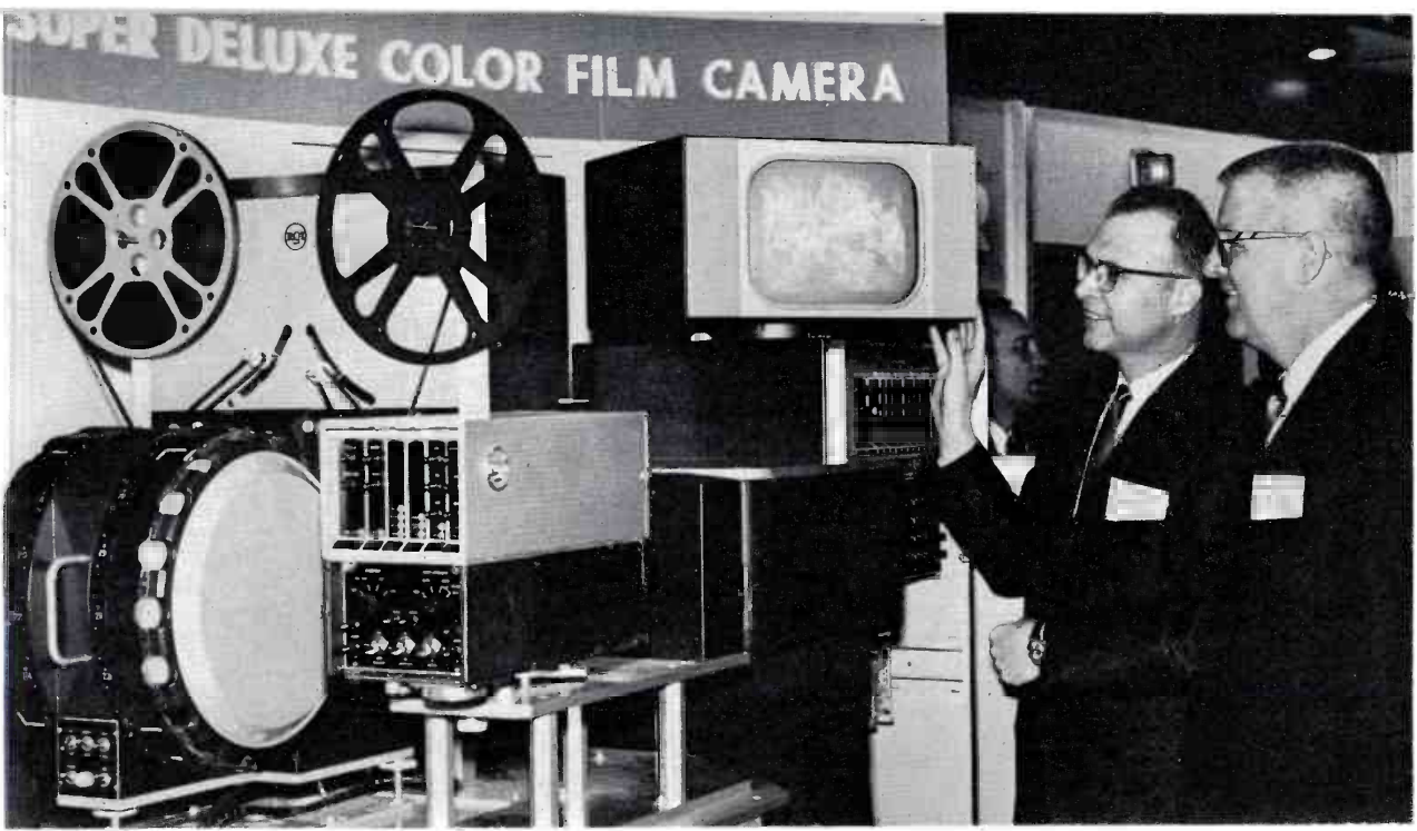
▲ COLOR FILM SYSTEM with a big difference—a 1½-inch vidicon tube in its luminance channel—is the subject of this operating display which produced show-stopping color film pictures. New Look equipments in the system pictured include TP-7 slide projector, TK-22 monochrome film camera, TP-66 film projector and TK-27 4-V color film camera.
