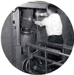
FIG. 9. Push release button; tilt tube.
