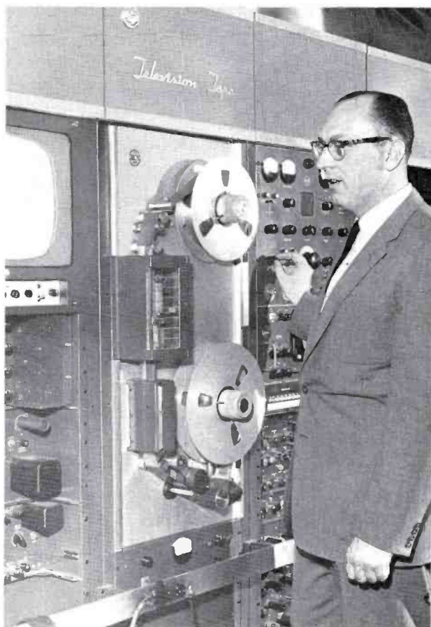
FIG. 1. Chief Engineer, Larry Larson, KSTP Television is shown operating one of the two new RCA TV Tape Recorders installed at KSTP-TV, Minneapolis/St. Paul.
