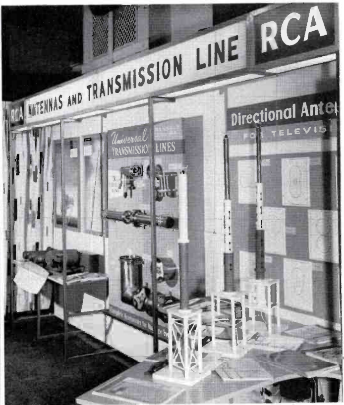
FIG. 10. Scale models of directional and traveling wave antennas are shown with typical patterns displayed on the rear wall. Universal transmission lines were shown next to these antennas. On the left a section of the BFA-series of FM antennas was displayed.
