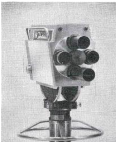
FIG. 3. New TK-12 Studio Camera is a logical teammate for tape. Featuring a 4½-inch image orthicon, it helps produce tape recording copies in greater number with greater detail.
