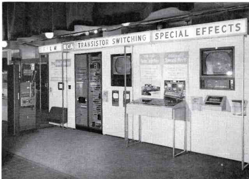
FIG. 5. The transistor switching and special effects display was set up so that broadcasters could actually perform switching operations and choose from the myriad of special effects patterns available in the equipment . . . wipes, split screens, picture insets, block, wedge, circular and multiple frequency patterns as well as a variety of keying effects.
