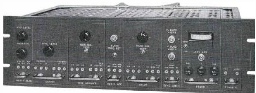
FIG. 8. The transistorized processing amplifier is housed on a single 5¼-inch rack mounted chassis which includes a self-contained d-c power supply. It is completely transistorized and combines many signal processing functions in one compact unit. It is comprised of eight plug-in modules to simplify test and maintenance.
