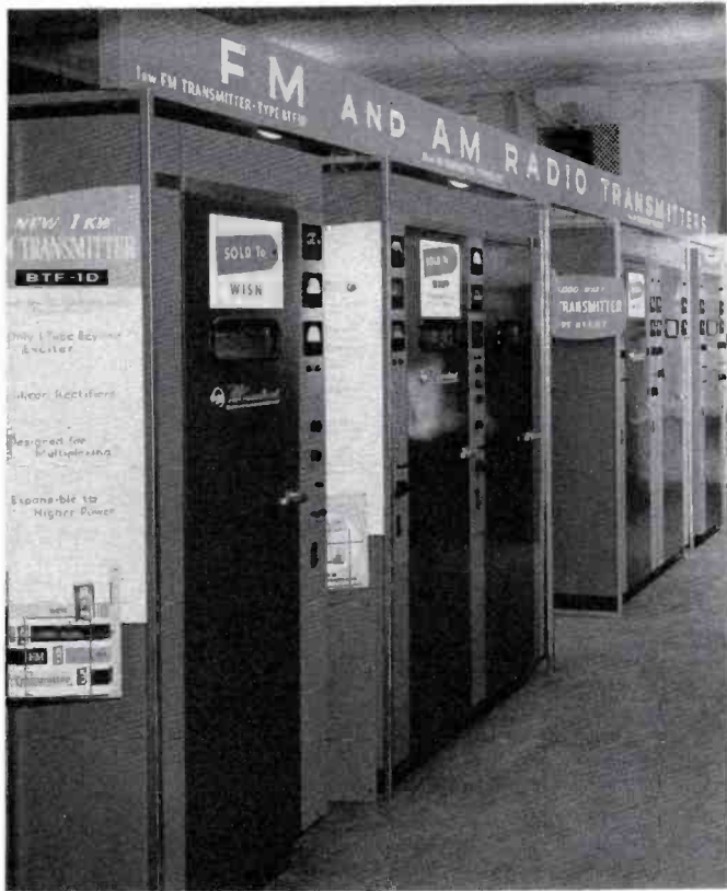
FIG. 9. Three new transmitters, shown from left to right, the BTF-1D 1-kw FM, the 10-kw BTF-10C FM, and the high efficiency 5-kw AM transmitter BTA-5T. At the end of the line is the old favorite BTA-1R, 1-kw AM transmitter.
