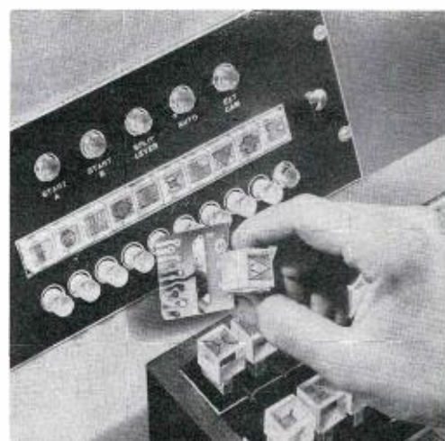
FIG. 4. Special effects equipment has been fully integrated into the system. Its use places a virtually unlimited range of effects at the producers fingertips—wipes, wedges, split screens, etc.
