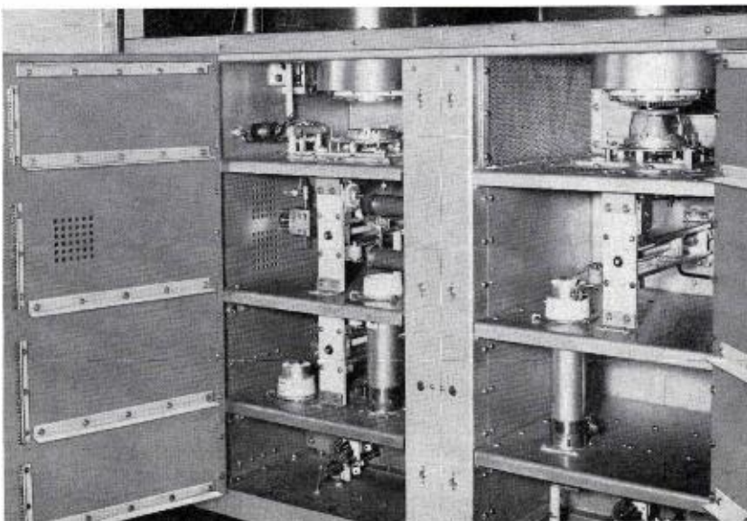
FIG. 5. This is the R-F Driver unit. The visual driver is shown on the left and the aural on the right. With panels open note ease of accessibility.
