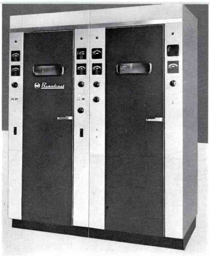
FIG. 1. Front view of BTA-5R. Easy access to all tubes and operating controls is made through the two interlocked front doors. The PA, modulator, and rectifier components are in the cabinet on the right, and the exciter, IPA, and control equipment are on the left. Attractive aluminized-steel cabinets provide improved shielding, and the doors are available in a choice of red, green, blue, or gray finishes.
