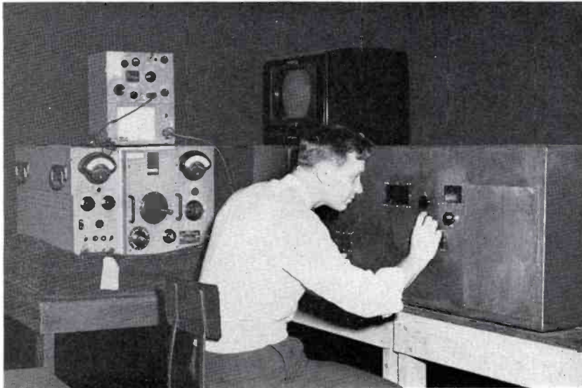
FIG. 4. Here author is shown running attenuation and propagation function tests on a TW antenna.
