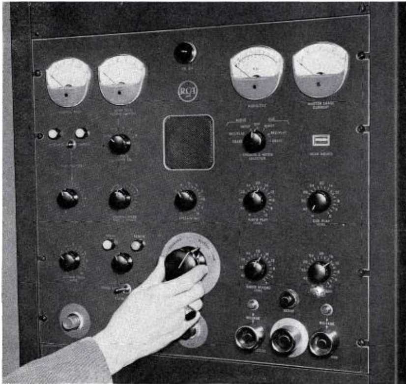
FIG. 5. Variable speed cuing control enables operators to rapid cue any point on the tape.
