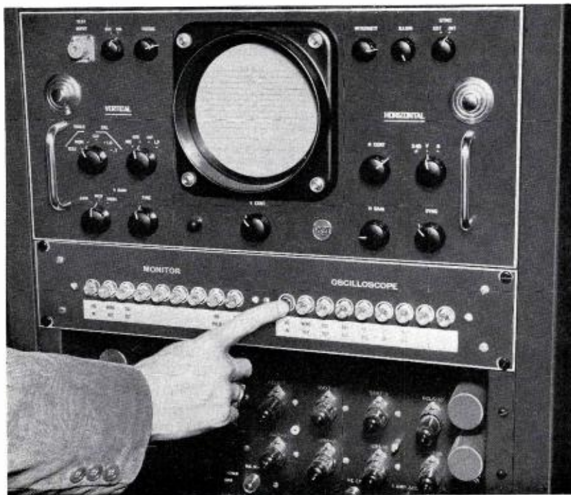
FIG. 8. Built-in switchers for monitor and oscilloscope permit instantaneous signal monitoring at key test positions.
