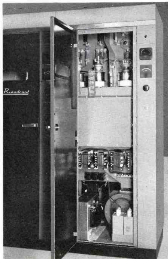
FIG. 3. The IPA and modulator driver stages are shown at the top of the opened cabinet. The exciter is at the center of the cabinet, and control equipment is placed just below it.
