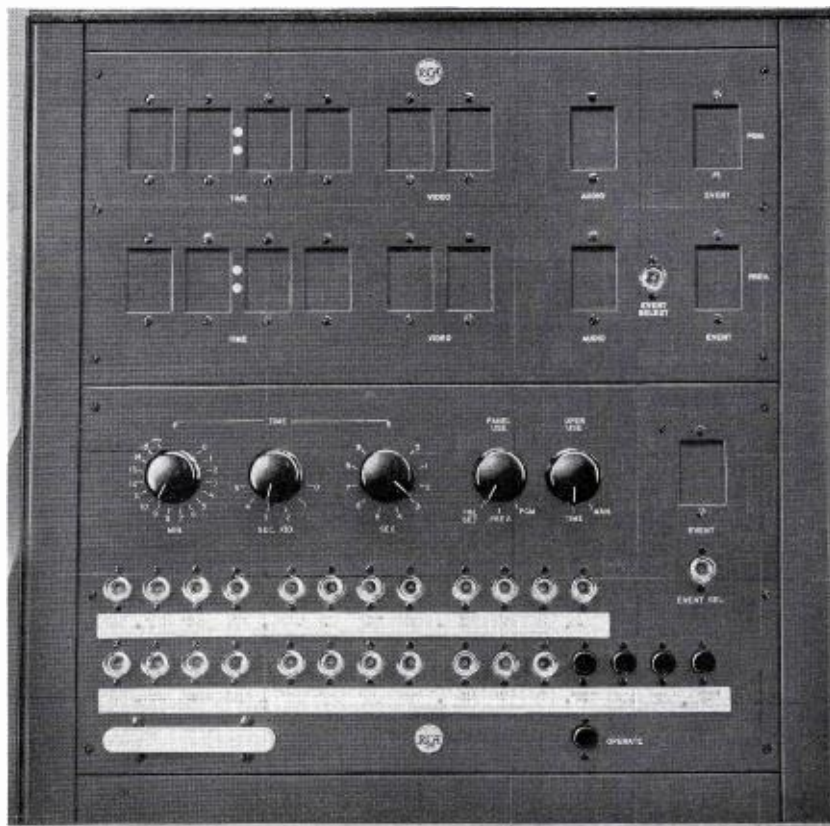
FIG. 3. Control and read-out panels of the TSA-1 system shown in the functional diagram Fig. 5.
