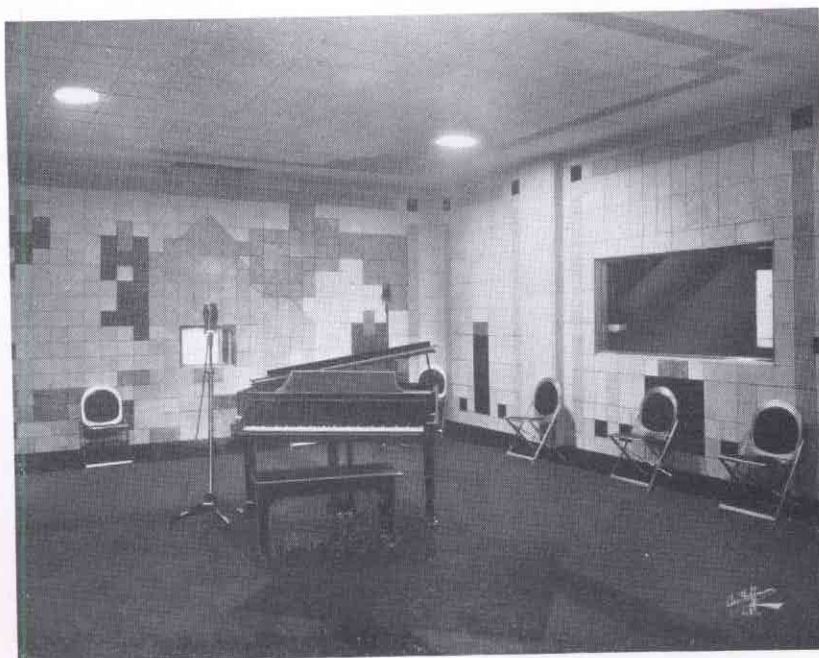
STUDIO A OF STATION WBRE, LOOKING INTO THE "DEAD END." VELOCITY MICROPHONE, ACOUSTIC WALL TREATMENT, AND INDIRECT LIGHTING HAVE CONTRIBUTED TO BRING THE LAST WORD IN MODERNIZATION INTO THESE STUDIOS.
