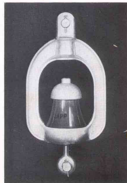
GUY INSULATORS USED TWO IN SERIES ON DIRECTIONAL BROADCAST ANTENNAE WFLA-WFSB IN BREAKING STRENGTH 90,000 LBS.
